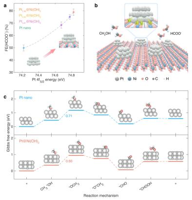
Fig. 4 Methanol e-refinery mechanisms towards formate. (a) The relationship between Pt 4f<sub>5/2</sub> energy and formate faradaic efficiencies of Pt<sub>x</sub>@Ni(OH)<sub>2</sub> (x = 1.05, 3.00, and 4.91) and Pt nano. (b) The reaction diagram of methanol e-refinery on Pt-loaded Ni(OH)<sub>2</sub>. (c) Possible reaction route and the corresponding computed free energy changes of methanol e-refinery towards formate on Pt and Pt-loaded Ni(OH)<sub>2</sub>
