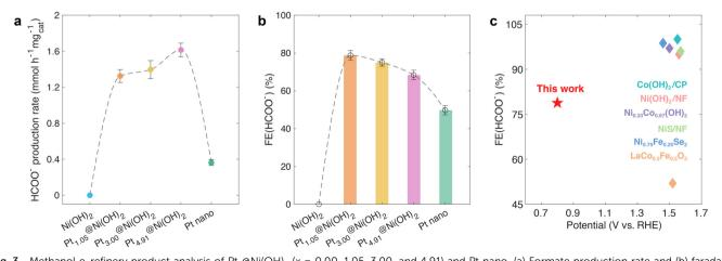
Fig. 3 Methanol e-refinery product analysis of  $Pt_x@Ni(OH)_2$  (x = 0.00, 1.05, 3.00, and 4.91) and Pt nano. (a) Formate production rate and (b) faradaic efficiency. (c) Performance comparison between Pt<sub>1.05</sub>@Ni(OH)<sub>2</sub> and other methanol e-refinery catalysts in the literature.
