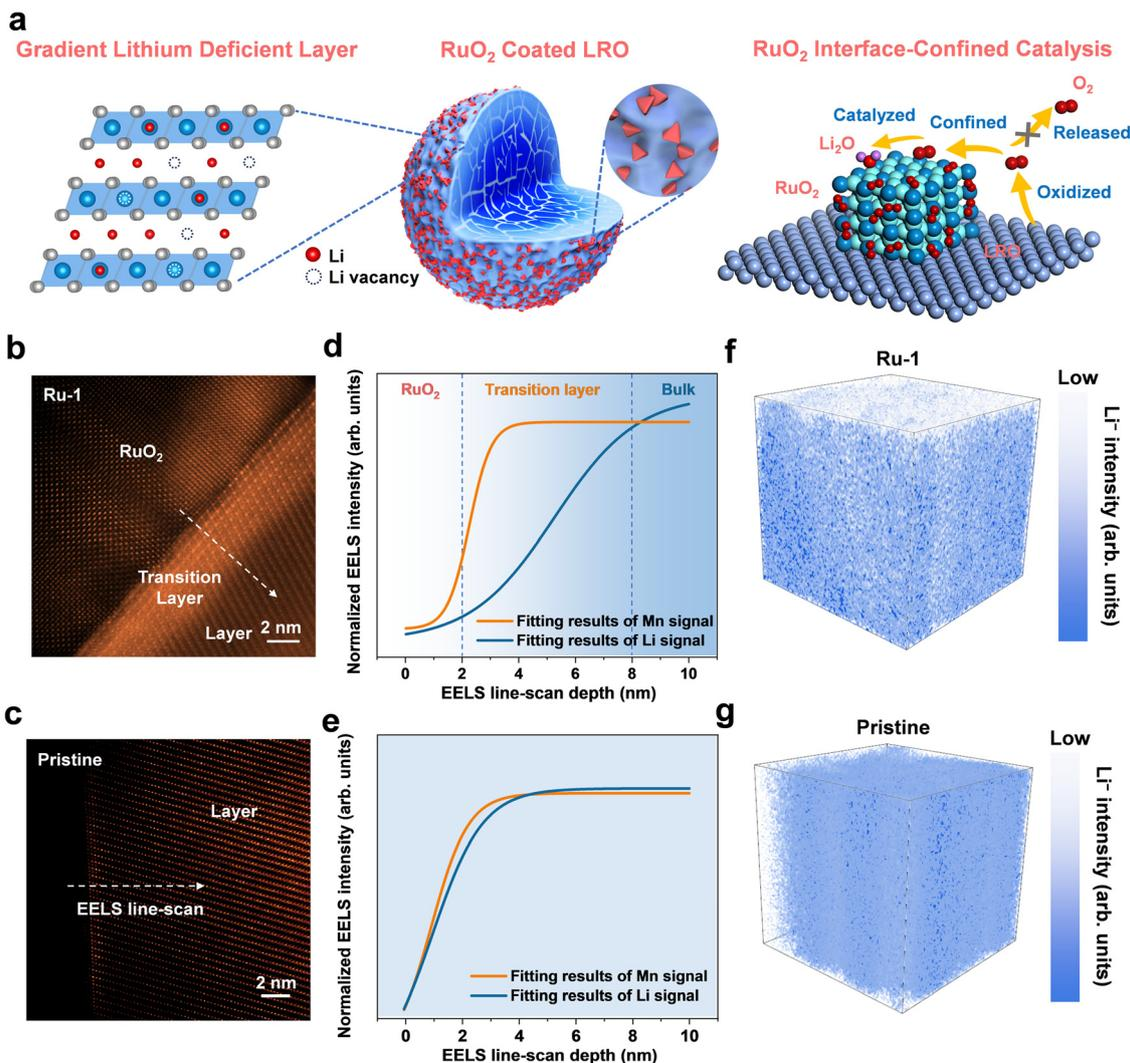
**Fig. 1** (a) Schematic diagram of the gradient lithium-deficient layer and  $\text{RuO}_2$  interface-confined catalysis in Ru-1. Characterization of a lithium-deficient layer. HAADF-STEM images of (b) Ru-1 and (c) the pristine sample. The normalized EELS intensities of the line-scan from the surface to the bulk of (d) Ru-1 and (e) pristine samples. The 3D plots of the TOF-SIMS  $\text{Li}^-$  intensity of (f) Ru-1 and (g) pristine samples. The blue region corresponds to the high Li content.
