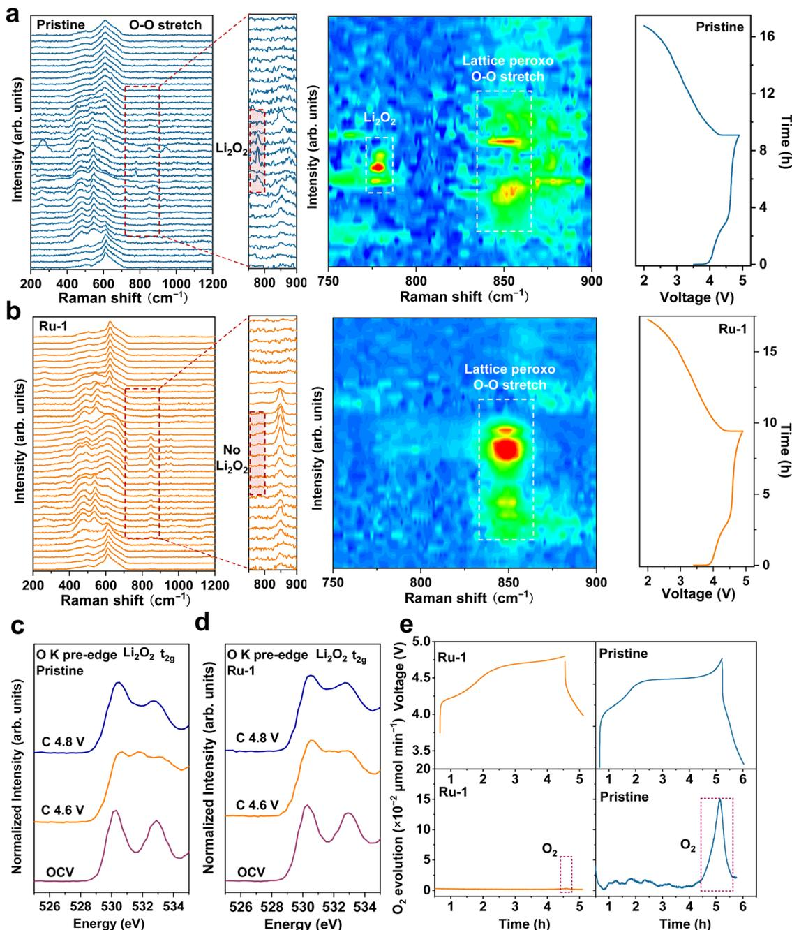
Fig. 2 Lattice oxygen stability comparison between Ru-1 and the pristine sample. Spectra and contour plots of the *in situ* SRES tests and the corresponding charge and discharge curves of (a) pristine sample and (b) Ru-1. The XAS O K-edge spectra of (c) the pristine sample and (d) Ru-1. (e) DEMS spectra and the corresponding charge curves of Ru-1 and the pristine sample.
