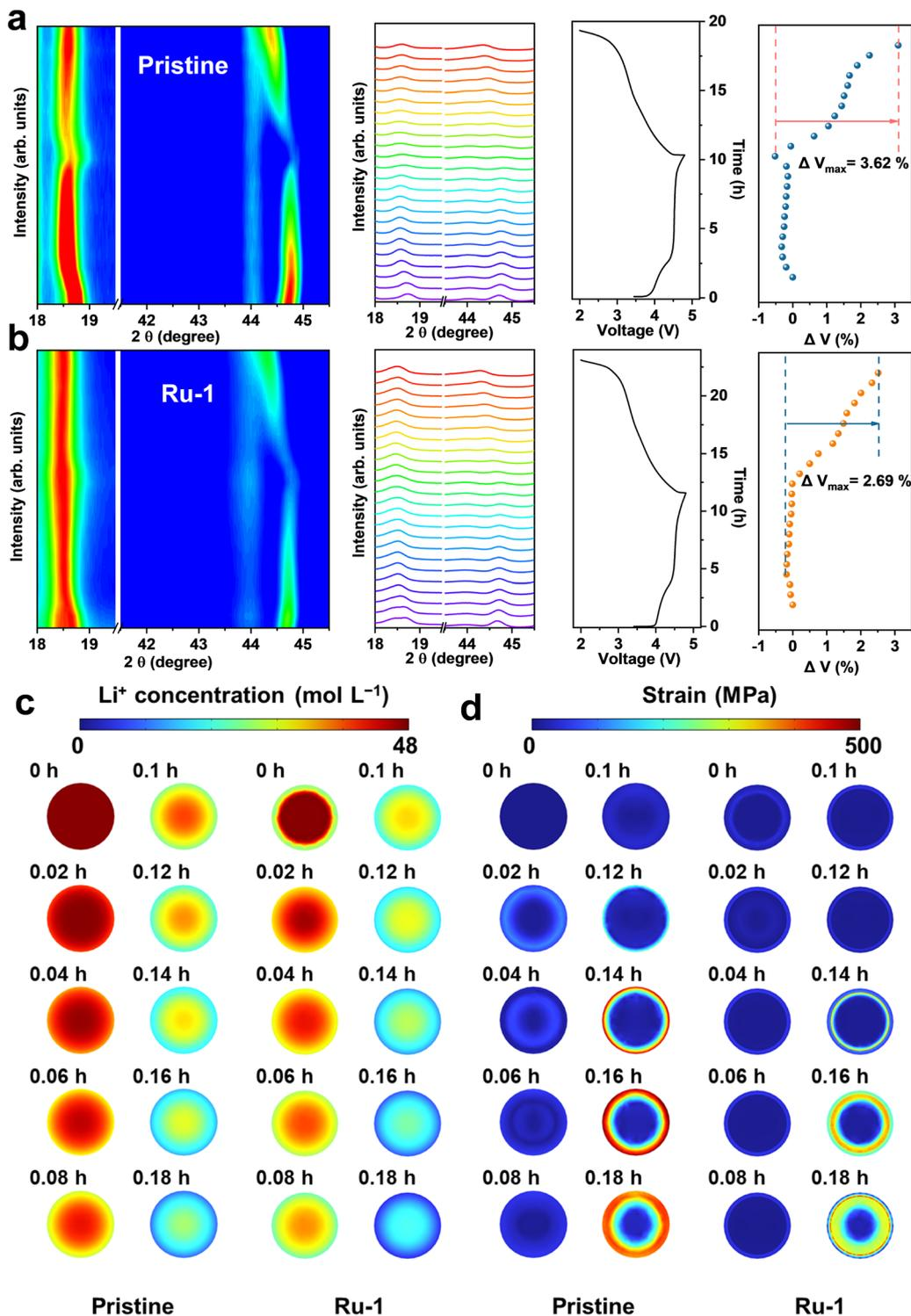
Fig. 4 Strain changes during the electrochemical process. The contour plots and spectra of the *in situ* XRD results and the corresponding volume changes of (a) the pristine sample and (b) Ru-1. The volume data are derived from GSAS software. Visualization of the (c) concentration and (d) strain changes during the initial charge process.
