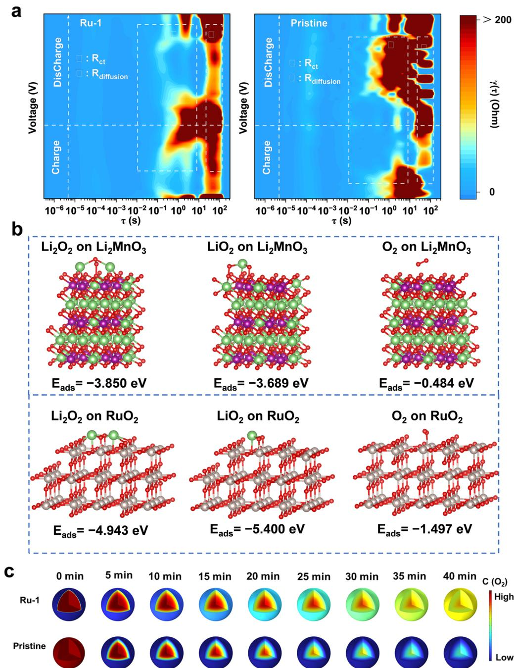
Fig. 6 The adsorption and catalytic capability evaluation. (a) DRT profile transformation from GEIS of Ru-1 and the pristine sample. (b) The models and adsorption energies of  $Li_2O_2$ ,  $LiO_2$ , and  $O_2$  adsorbed on  $Li_2MnO_3$  and  $RuO_2$ . (c)  $O_2$  diffusion simulation of Ru-1 and the pristine sample with COMSOL software.
