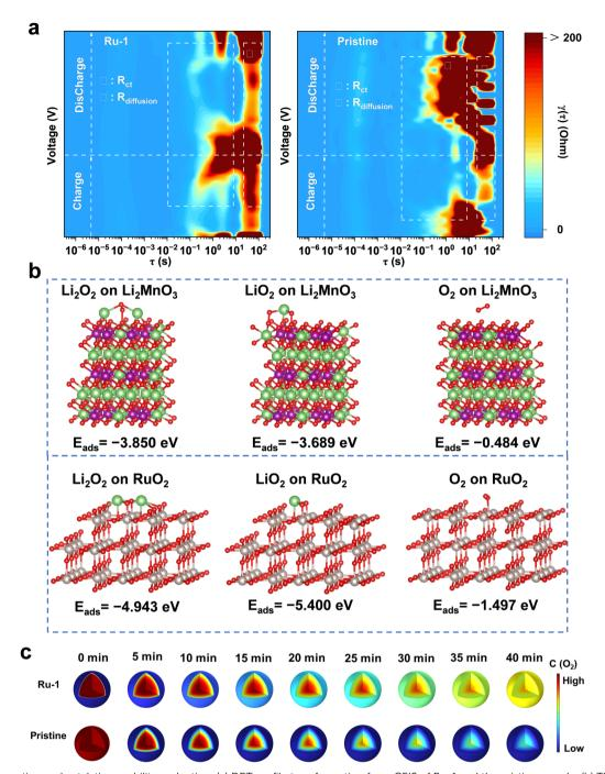
Fig. 6 The adsorption and catalytic capability evaluation. (a) DRT profile transformation from GEIS of Ru-1 and the pristine sample. (b) The models and adsorption energies of Li<sub>2</sub>O<sub>2</sub>, LiO<sub>2</sub>, and O<sub>2</sub> adsorbed on Li<sub>2</sub>MnO<sub>3</sub> and RuO<sub>2</sub>. (c) O<sub>2</sub> diffusion simulation of Ru-1 and the pristine sample with COMSOL software.
