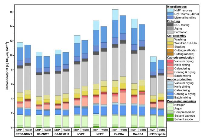
Fig. 7 CF of prismatic cell production for selected SIB cell chemistries in the HC-basic scenario compared to LFP/graphite cells, distinguishing between NMP-based and aqueous cathode processing. Wel. = welding, Pac. = packaging; Fil. = electrolyte filling, Clo. = closing, EOL = end of line.
