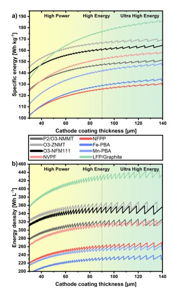
Fig. 4 Specific energy (a) and energy density (b) for selected SIB cell chemistries in the prismatic cell, HC-basic scenario depending on the cathode coating thickness, compared to an LFP/graphite cell. For Fe-PBA and Mn-PBA the electrochemical data from Altris/Northvolt and CATL are applied (cell 13 and 15 from Fig. 3). In this study the coating thickness was set to 90 µm, which is marked for clarification.
