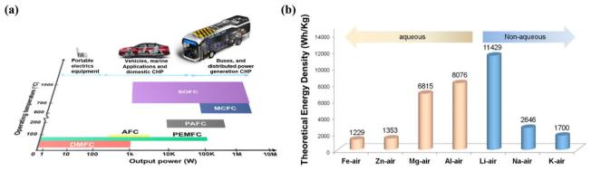
Fig. 2 Comparison of fuel cells and metal-air batteries: performance and energy density. (a) The relationship between the operating temperature and output power for several fuel cells. Copyright 2023, Elsevier. (b) Theoretical energy densities for different types of metal-air batteries. Copyright 2017, American Chemical Society
