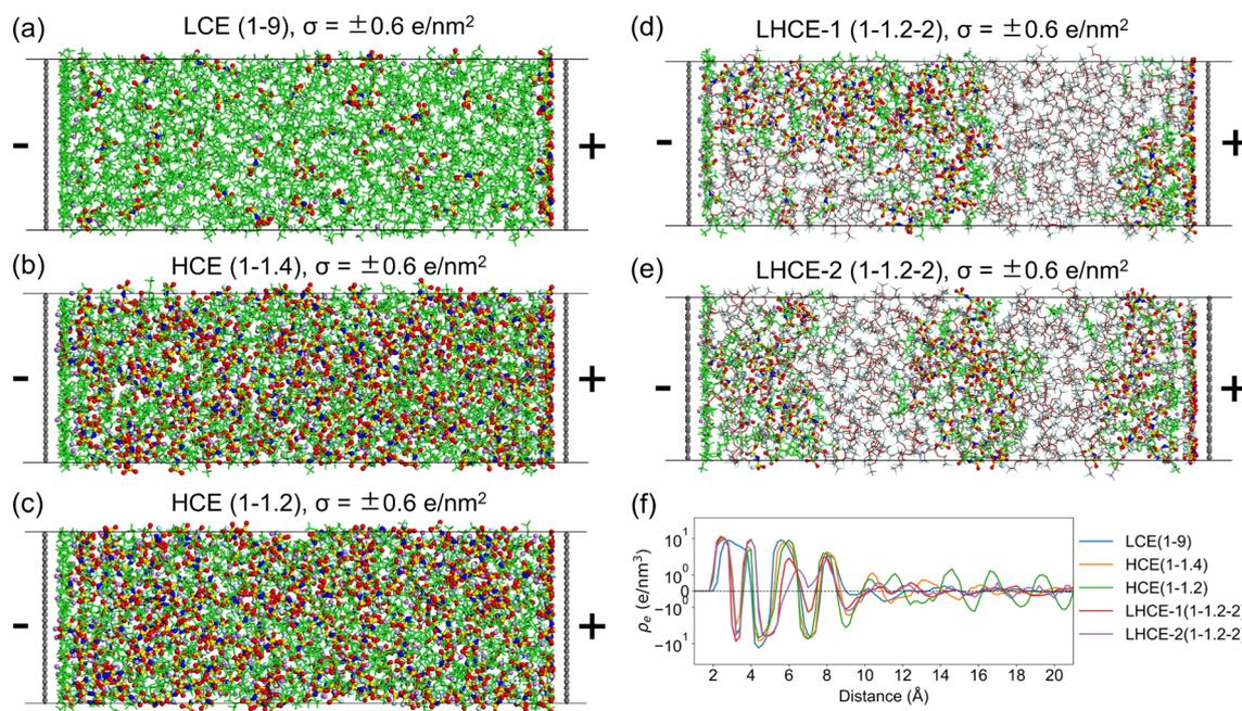
Fig. 3 Final frames of the MD trajectories for (a) LCE(1-9), (b) HCE(1-1.4), (c) HCE(1-1.2), and (d) and (e) LHCE(1-1.2-2) under a graphene surface charge density of  $\sigma = \pm 0.6 \text{ e nm}^{-2}$ . (f) Charge density profiles (as a function of distance from the negatively charged graphene electrode; in a symmetric logarithmic plot) of the LCE, HCE, and LHCE systems.
