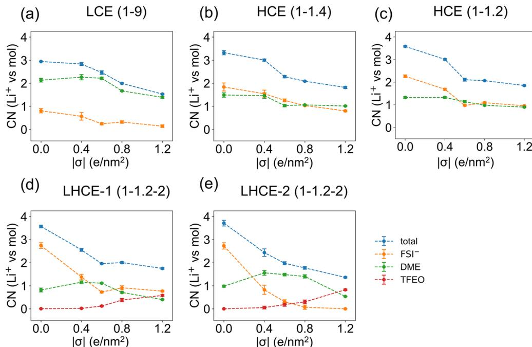
Fig. 6 Coordination numbers between the first-layer Li<sup>+</sup> ions in the EDL (within 5.0 Å from the negatively charged graphene electrode) and other species (FSI<sup>-</sup>, DME, and TFEO) under different surface charge densities of the graphene electrode for (a) LCE(1-9), (b) HCE(1-1.4), (c) HCE(1-1.2), (d) LHCE-1(1-1.2-2), and (e) LHCE-2(1-1.2-2).
