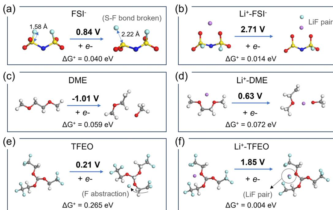
Fig. 7 DFT-optimized geometries of the redox species and calculated reduction potentials for (a) FSI<sup>-</sup>, (b) LiFSI, (c) DME, (d) Li<sup>+</sup>-DME, (e) TFEO, and (f) Li<sup>+</sup>-TFEO. The gray, red, white, purple, light blue, yellow, and dark blue spheres stand for C, O, H, Li, F, S, and N atoms, respectively. Reduction reaction barriers are calculated following Nelsen's four-point method.<sup>53</sup>
