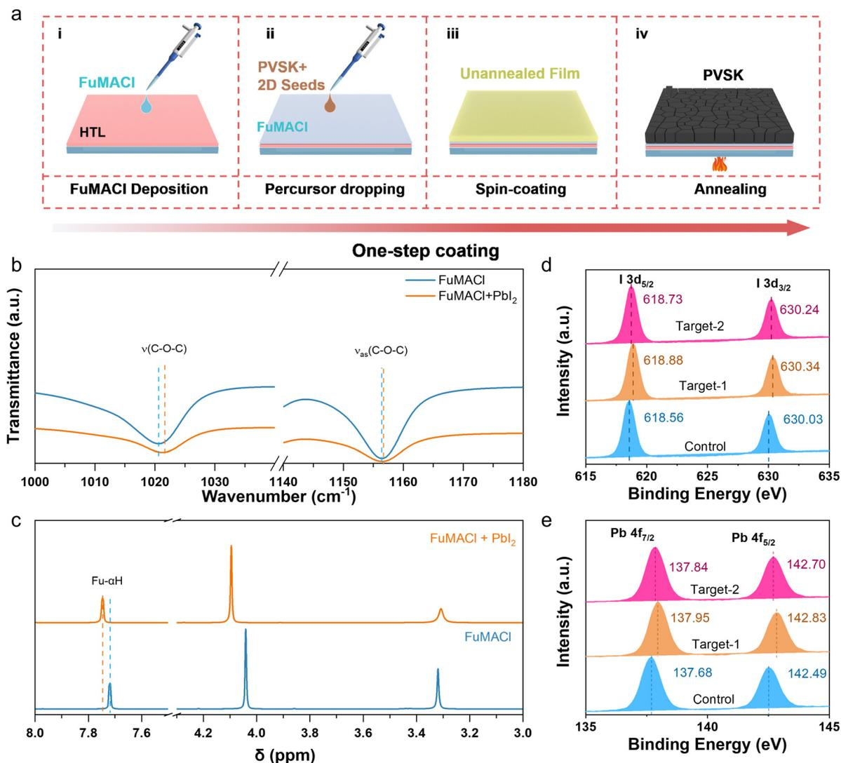
**Fig. 1** (a) Process diagram of the one-step spin-coating method for preparing target perovskite films. (b) FTIR spectra of FuMACl and FuMACl/PbI<sub>2</sub> complex. (c) Chemical shift information of FuMACl and FuMACl/PbI<sub>2</sub> complex obtained from <sup>1</sup>H NMR measurements. (d) and (e) XPS spectra of the control, target-1 and target-2 perovskite films.
