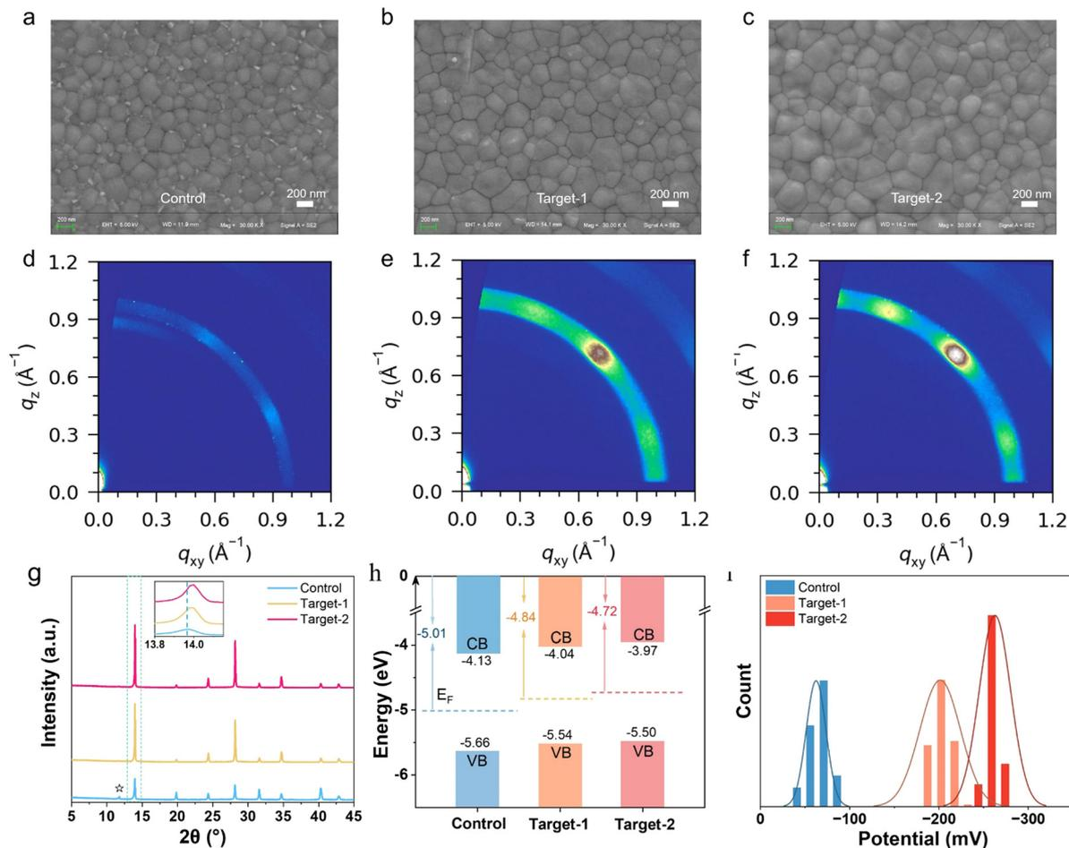
Fig. 3 (a) Top-view SEM image of the control film. (b) Top-view SEM image of the target-1 film. (c) Top-view SEM image of the target-2 film. (d)–(f) GIWAXS patterns of the control, target-1 and target-2 films. (g) XRD patterns of the control, target-1 and target-2 perovskite films. (h) Energy-level diagrams of the perovskite films. (i) KPFM of the control, target-1 and target-2 perovskite films.
