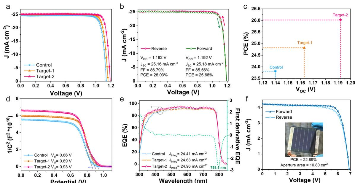
Fig. 4 (a)  $J$ - $V$  curves of the control, target-1 and target-2 devices under reverse scan. (b)  $J$ - $V$  curves of reverse and forward scans for the optimized target-2 device. (c) PCE and  $V_{oc}$  of the control, target-1 and target-2 devices. (d) Mott-Schottky plots for the corresponding devices. (e) EQE spectra of the corresponding devices. (f)  $J$ - $V$  curves of reverse and forward scans for the target-2 film based mini-module ( $10.80 \text{ cm}^2$ ).
