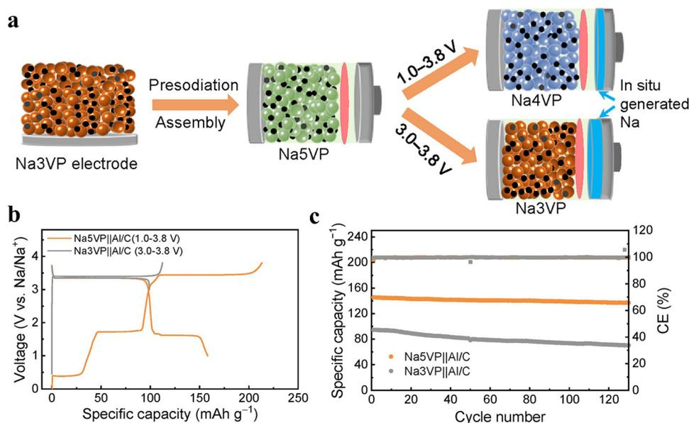
Fig. 17 (a) Illustration of presodiation, assembly, and operation of AFSMB in two different voltage windows, (b) initial GCD profiles and (c) cyclic performance of Na<sub>5</sub>VP||Al cells within different voltage windows (1.0–3.8 and 3.0–3.8 V). Reproduced with permission.<sup>31</sup> Copyright 2021 Wiley-VCH GmbH.
