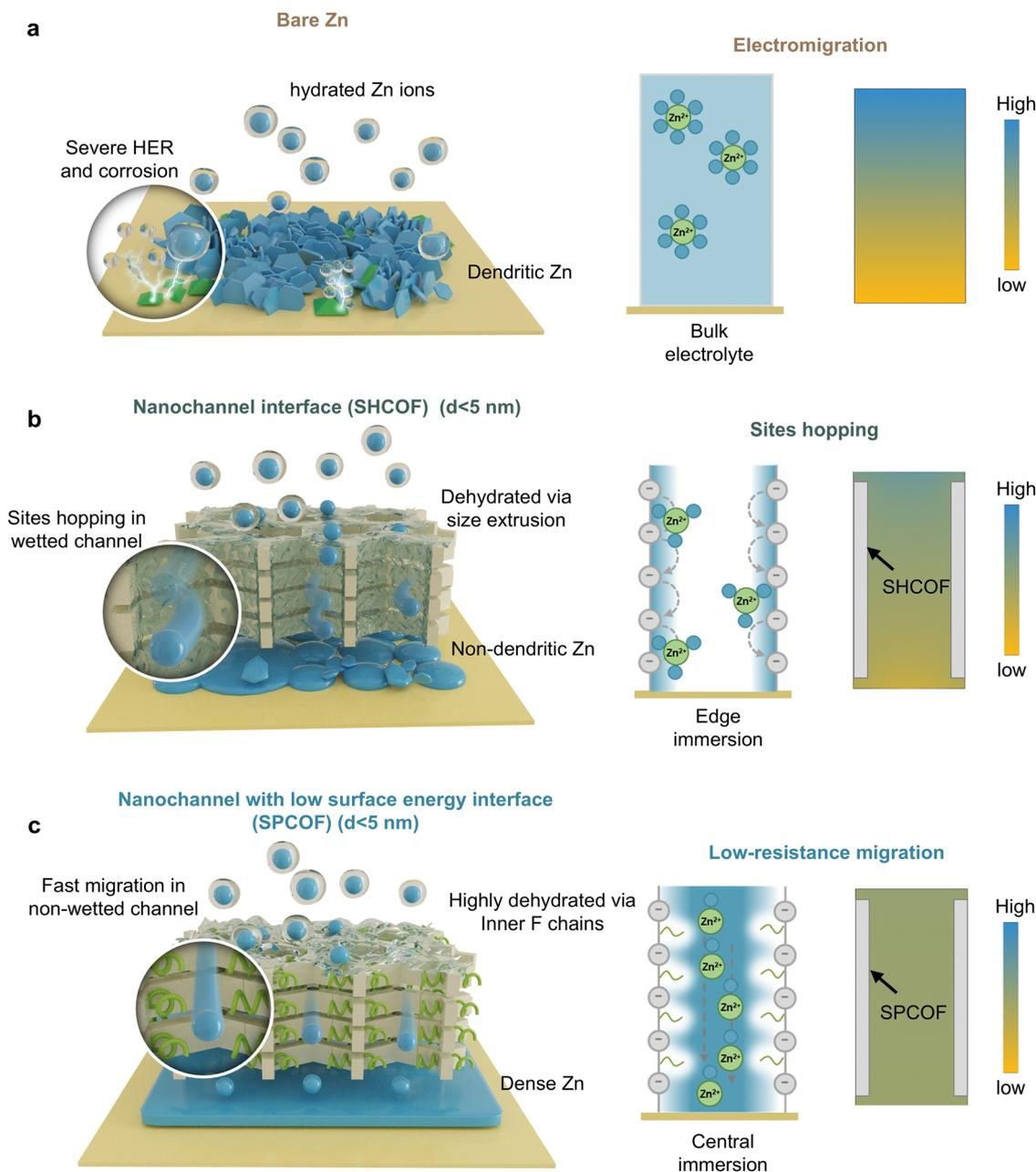
**Fig. 1** Schematic illustrations showing Zn interface with different interface. Schematic illustrations depicting various ion migration mechanisms and the Zn deposition process on different surfaces, along with the corresponding ion concentration profiles near the electrode surface simulated using COMSOL. (a) Bare Zn. (b) Zn with nanochannel interface ( $d < 5$  nm). (c) Low surface energy nanochannel interface ( $d < 5$  nm).
