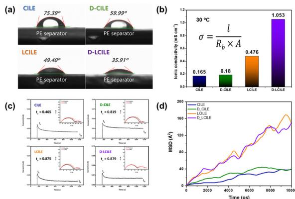
Fig. 3 Characteristics of ionic liquid-based electrolytes (CILE, D-CILE, LCILE, and D-LCILE): (a) wettability on PE separator, (b) ionic conductivity, (c) Li<sup>+</sup> transference number measured by Bruce–Vincent method, and (d) diffusion coefficient measured from MSD plot.
