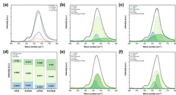
Fig. 1 Raman spectra in the 650–800  $\text{cm}^{-1}$  region: (a) CILE, D-CILE, LCILE, and D-LCILE; (d) free anion, CIP, and AGGs fractions; (b), (c), (e) and (f) peak deconvolutions of (b) CILE, (c) D-CILE, (e) LCILE, and (f) D-LCILE.
