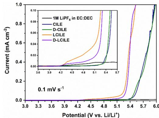
Fig. 4 Linear sweep voltammograms of Li||SS cells in 1 M LiPF<sub>6</sub> in EC:DEC (1:1, v/v), CILE, D-CILE, LCILE, and D-LCILE at a scan rate of 0.1 mV s<sup>-1</sup>.
