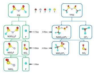
Dissociation mechanism of FSI and TFSI anions analyzed using
