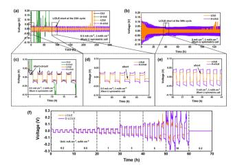
Fig. 8 Symmetric cell test with 20 µm-thick Li: (a) voltage profiles in CILE, D-CILE, LCILE, and D-LCILE at 0.5 mA cm<sup>-2</sup> and 1 mA h cm<sup>-2</sup>, (b) voltage profiles in LCILE and D-LCILE at 3 mA cm<sup>-2</sup> and 1 mA h cm<sup>-2</sup>, (c) first five cycles, (d) five cycles after 80 hours at 0.5 mA  $cm^{-2}$  and 1 mA h  $cm^{-2}$ , and (e) eight cycles after 36 h at 3 mA cm $^{-2}$  and 1 mA h cm $^{-2}$ , (f) critical current density measurements of LCILE and D-LCILE
