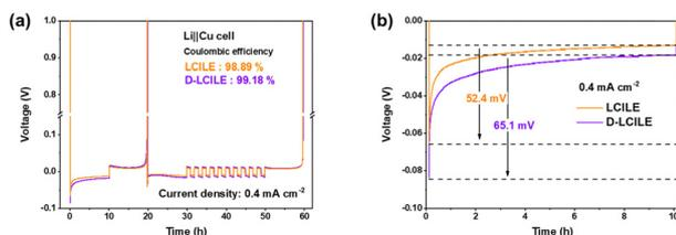
Fig. 5 Electrochemical performance of LCILE and D-LCILE in a Li||Cu cell configuration: (a) average coulombic efficiency for LCILE and D-LCILE measured by the advanced Aurbach method at 0.4 mA cm<sup>-2</sup>, and (b) voltage overpotential at 0.4 mA cm<sup>-2</sup>.
