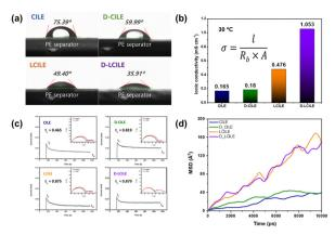
Fig. 3 Characteristics of ionic liquid-based electrolytes (CILE, D-CILE, LCILE, and D-LCILE): (a) wettability on PE separator, (b) ionic conductivity, (c) Li<sup>+</sup> transference number measured by Bruce-Vincent method, and (d) diffusion coefficient measured from MSD plot.
