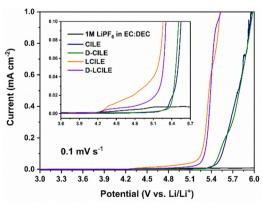
Fig. 4 Linear sweep voltammograms of Li||SS cells in 1 M LiPF<sub>6</sub> in EC:DEC (1:1, v/v), CILE, D-CILE, LCILE, and D-LCILE at a scan rate of  $0.1 \text{ mV s}^{-1}$ .
