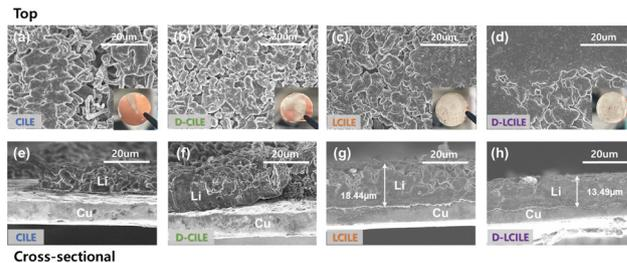
Fig. 6 SEM images of Li plated on a Cu substrate in different electrolytes at a current density of 1 mA cm<sup>-2</sup> and an areal capacity of 1 mA h cm<sup>-2</sup>: (a)–(d) top-view images and (e)–(h) cross-sectional images.
