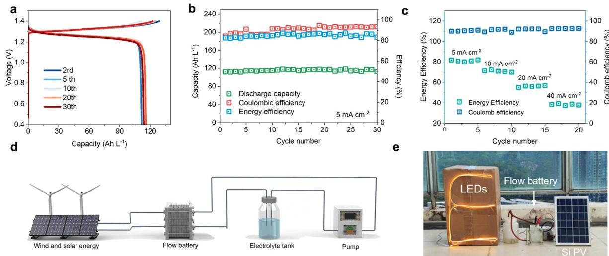
**Fig. 5** Proof-of-concept membrane-free flow battery based on the DPZIB. (a) GCD curves, (b) cycling performance and (c) rate capability. (d) Schematic illustration of the integration of membrane-free DPZIB flow battery in grid-scale energy storage system, and (e) a prototype that continuously powers a LED light chain (5 W).
