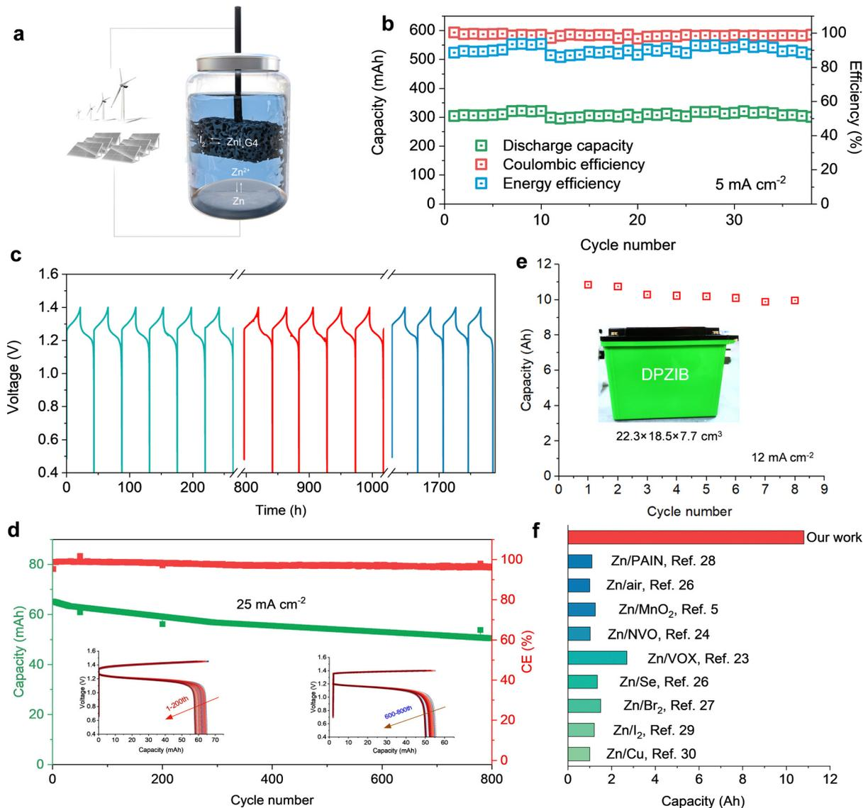
Fig. 4 Electrochemical performance of the DPZIB. (a) Schematic illustration of the configuration of the DPZIB. (b) Cycling performance and (c) time–voltage curves of DPZIB at a current of  $5 \text{ mA cm}^{-2}$ . (d) Long cycling performance of the DPZIB. (e) Capacity of a large-sized static DPZIB and (f) comparison to various aqueous batteries.
