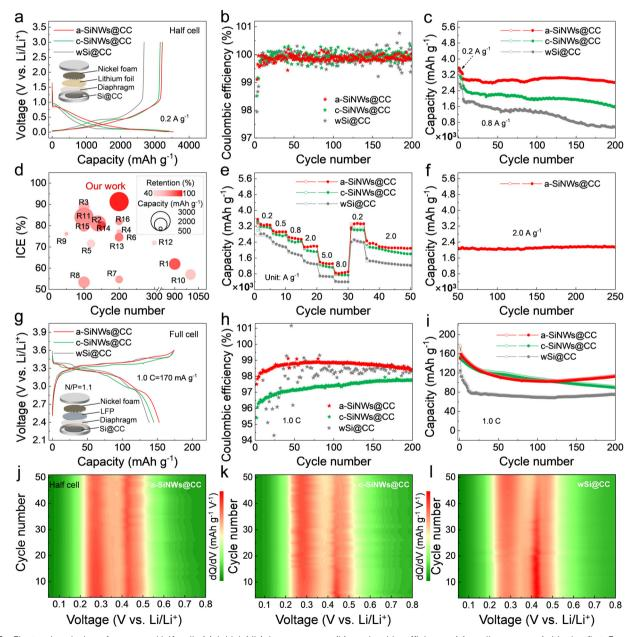
Fig. 5 Electrochemical performance. Half cell: (a) initial (dis)charge curves, (b) coulombic efficiency, (c) cycling curves (with the first 3 cycles at 0.2 A  $g^{-1}$ ), (d) comparison with the recently reported Si nanowire electrodes, (e) rate curves, and (f) cycling curves (continuing from Fig. 5e). Full cell: (g) initial (dis)charge curve, (h) coulombic efficiency, (i) cycling curves and (j)–(l) differential capacity (dQ/dV) versus voltage contour plots.
