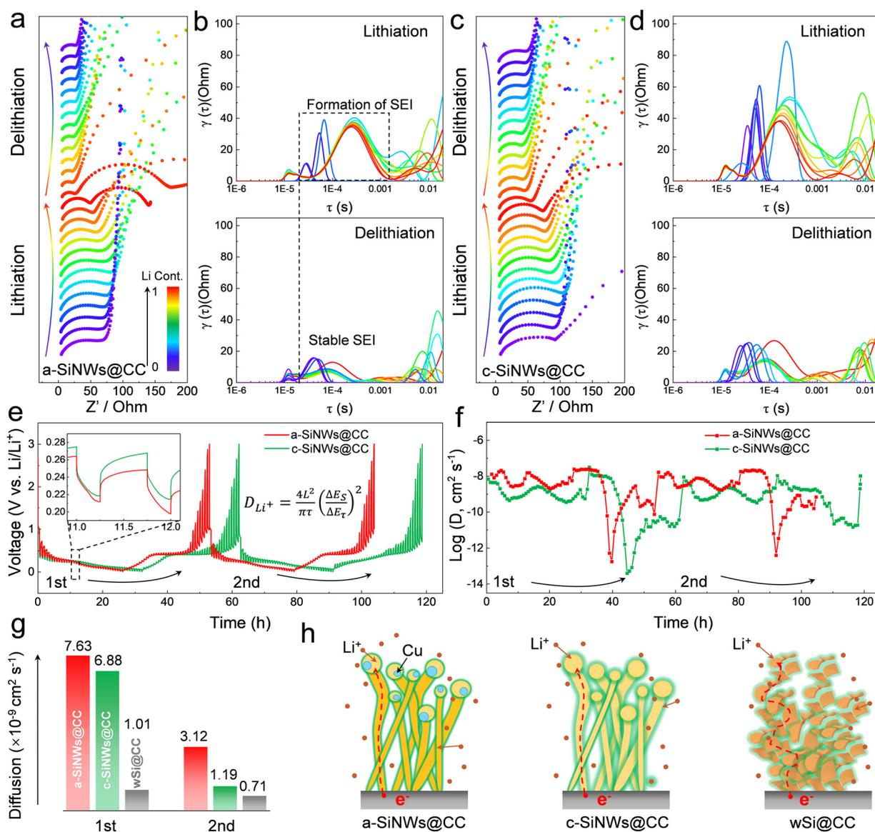
Fig. 6 Kinetic properties. *In situ* EIS and corresponding DRT of (a) and (b) a-SiNWs@CC and (c) and (d) c-SiNWs@CC during the first (de)lithiation, (e) and (f) GITT test, (g) apparent ion diffusion values for the electrodes, and (h) schematic diagram of ion transport pathways and interface stability for different electrodes.
