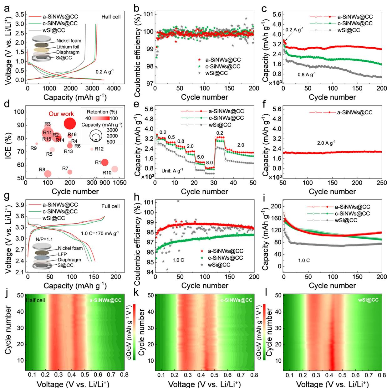
Fig. 5 Electrochemical performance. Half cell: (a) initial (dis)charge curves, (b) coulombic efficiency, (c) cycling curves (with the first 3 cycles at  $0.2 \text{ A g}^{-1}$ ), (d) comparison with the recently reported Si nanowire electrodes, (e) rate curves, and (f) cycling curves (continuing from Fig. 5e). Full cell: (g) initial (dis)charge curve, (h) coulombic efficiency, (i) cycling curves and (j)–(l) differential capacity ( $dQ/dV$ ) versus voltage contour plots.
