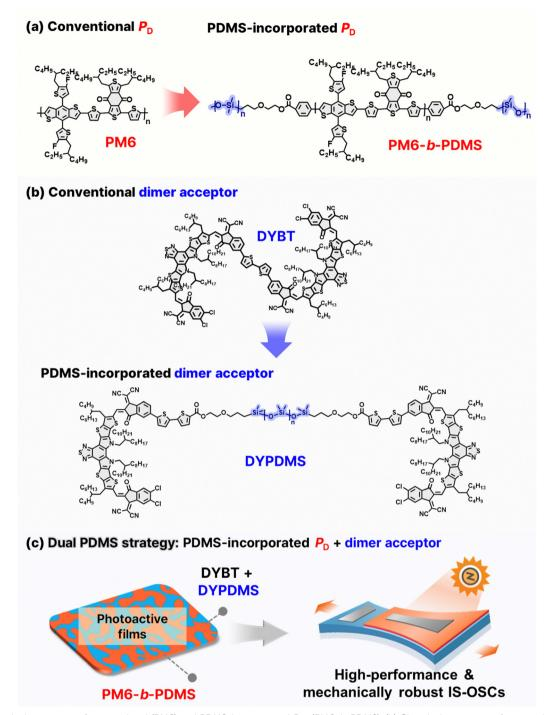
Fig. 1 (a) Chemical structures of conventional (PM6) and PDMS-incorporated PDS (PM6-b-PDMS). (b) Chemical structures of conventional (DYBT) and PDMS-incorporated dimer acceptors (DYPDMS). (c) Conceptual illustration of the dual PDMS incorporation strategy to achieve enhanced mechanical robustness and photovoltaic performance in IS-OSCs.
