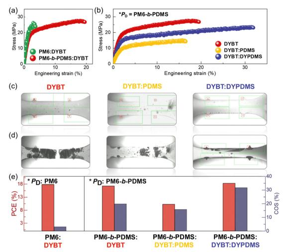
Fig. 4 (a) and (b) S-S curves of blend films for (a) P<sub>D</sub>:DYBT and (b) PM6-b-PDMS:acceptors, (c) and (d) OM images of the of PM6-b-PDMS:acceptors based blend films at (c) 0% and (d) 20% strain. (e) comparison of PCE and COS values among the photoactive systems studied.
