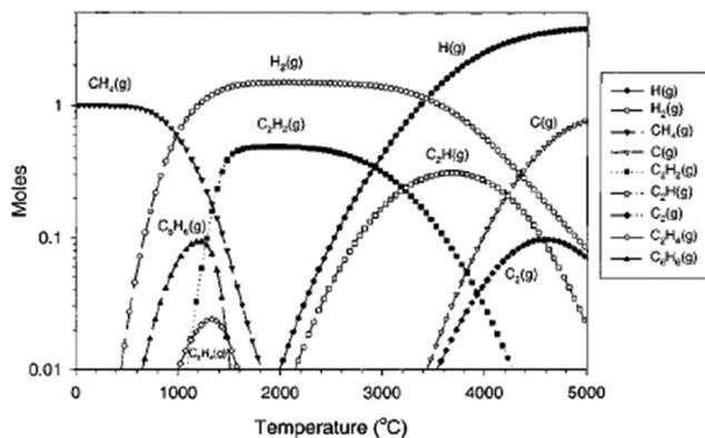
Fig. 18 Equilibrium diagram for decomposition of 1 mol of methane versus temperature including carbon, Reproduced from ref. 206 with permission from the American Chemical Society (open access), copyright 2002.
