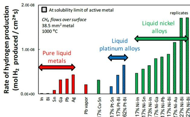
Fig. 21 The activity of different pure metals and alloys for the methane pyrolysis process. Adapted from ref. 249 with permission from The American Association for the Advancement of Science, copyright 2017.
