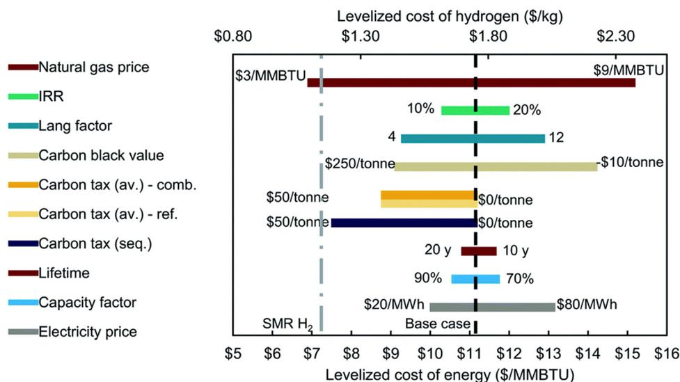
Fig. 26 The impact of feed cost, internal rate of return (IRR), lang factor, carbon sale, carbon tax, lifetime, capacity, and electricity cost on the LCOH for small-scale hydrogen production, reproduced from ref. 57 with permission from the Royal Society of Chemistry, copyright 2020.
