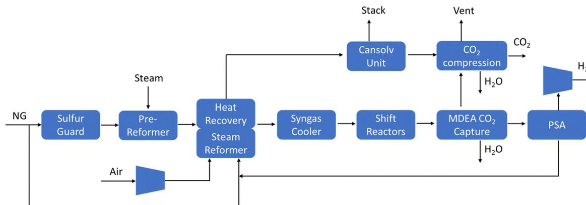
Fig. 2 Block flow diagram of a Steam Methane Reforming Plant with CO<sub>2</sub> capture. Source: adapted from reference (DOE Public Access).<sup>12</sup>
