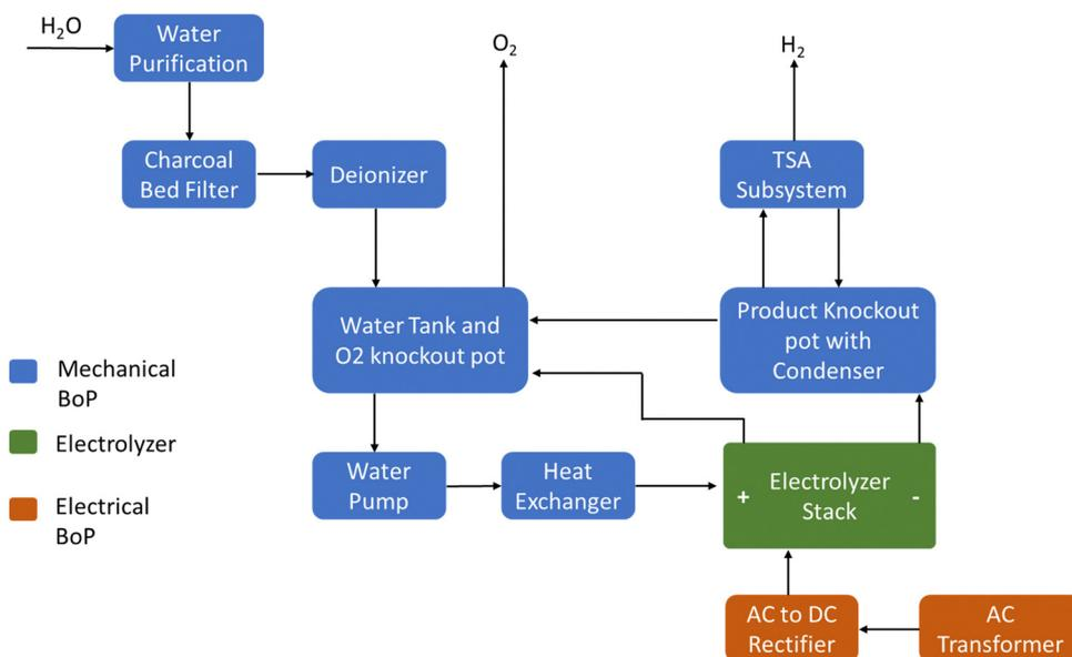
Fig. 3 Block flow diagram of PEM water electrolysis plant. Source: adapted from reference (DOE Public Access).<sup>20</sup>
