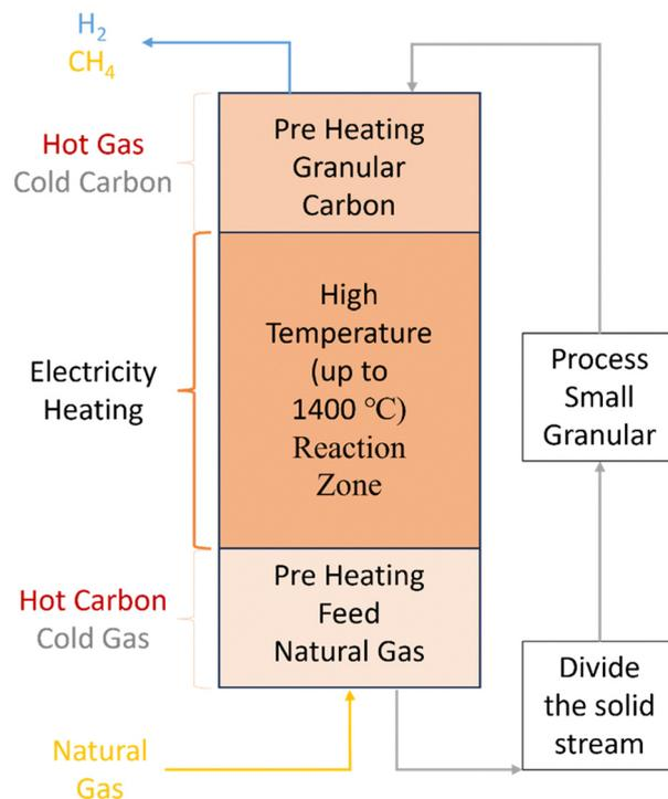
Fig. 14 Moving-bed reactor schematic and flows.<sup>152</sup>
