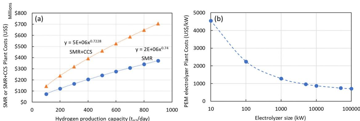
Fig. 4 (a) Plant costs (2020 US\$) for SMR or SMR + CCS plants versus plant size ( $\text{kg}_{\text{H}_2}$  per day) production (b) plant costs (2020 US\$) for PEM electrolyzers versus electrolyzer size (kW).
