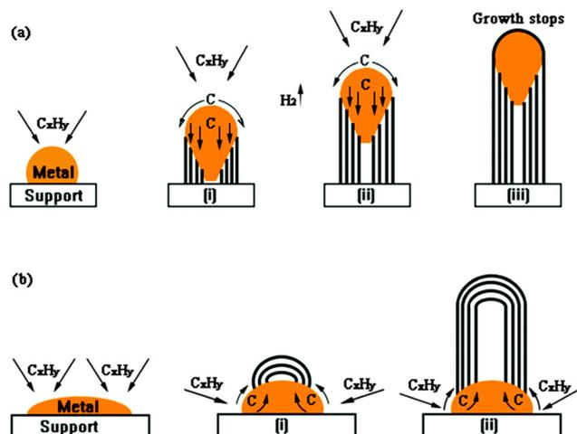
Fig. 24 Two types of carbon nanotubes deposition mechanisms including (a) tip-growth mechanism and (b) base-growth mechanism, Reproduced from ref. 294 with permission from the Royal Society of Chemistry, copyright 2015.
