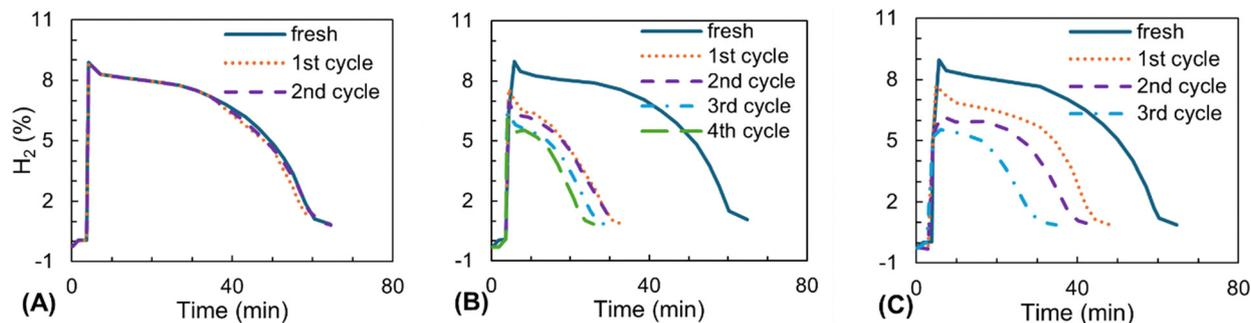
Fig. 12 The activity of Cu/Al<sub>2</sub>O<sub>3</sub> in producing H<sub>2</sub> in fresh and after regenerated by (A) air, (B) CO<sub>2</sub>, and (C) steam. Adapted from ref. 129 with permission from Taylor & Francis, copyright 2008.
