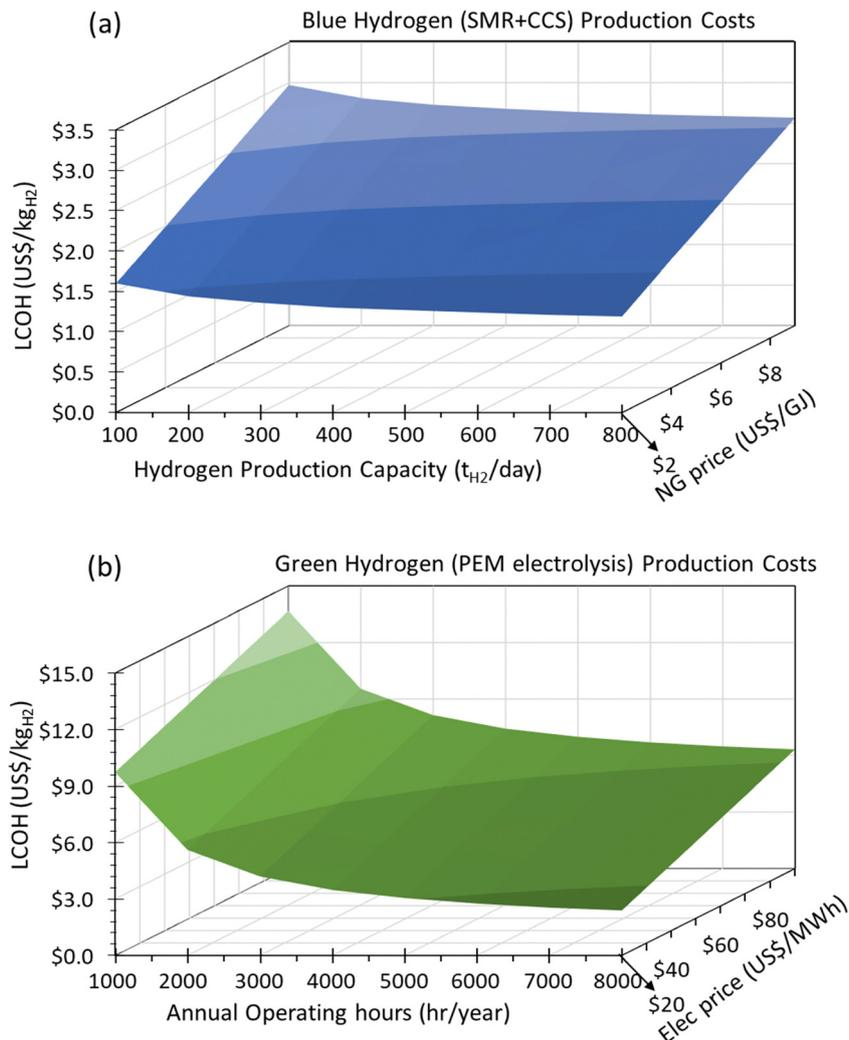
Fig. 5 (a) Levelized cost of blue hydrogen (\$ per  $\text{kg}_{\text{H}_2}$ ) produced via SMR + CCS as a function of natural gas price (\$ per GJ) and plant size ( $t_{\text{H}_2}$  per day). (b) Levelized cost of green hydrogen (\$ per  $\text{kg}_{\text{H}_2}$ ) produced via PEM electrolysis as a function of electricity price (\$ per MWh) and annual operating hours (hours per year).
