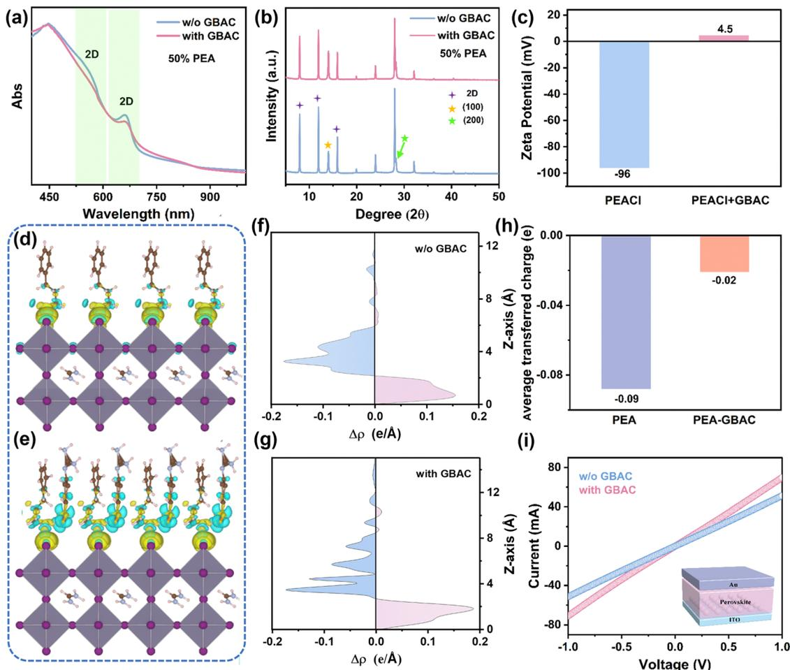
**Fig. 1** (a) UV-vis absorption spectra of tin perovskite films without and with GBAC. (b) XRD patterns of films without and with GBAC. (c) Zeta potentials of PEA solutions with and without GBAC. The electron density distribution of  $\text{FASnI}_3$  interacting with (d) PEA and (e) PEA-GBAC. (f) and (g) The charge transfer differences along the Z-axis, and (h) the average transferred charge. (i) The current–voltage ( $I$ – $V$ ) curves of devices without and with GBAC.
