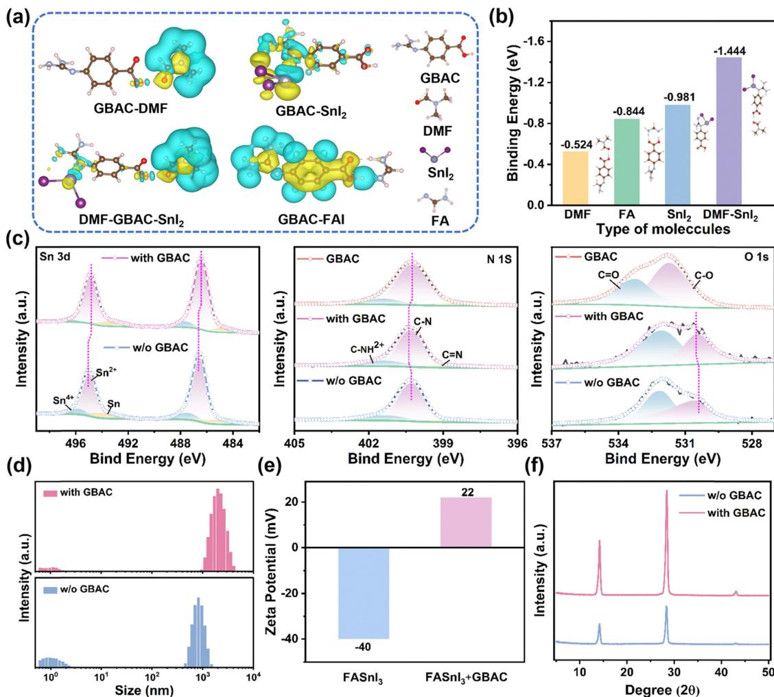
Fig. 3 (a) Distributions of the charge density from DFT and (b) binding energies of DMF, FAI,  $\text{SnI}_2$ , and  $\text{DMF-SnI}_2$  with GBAC, respectively. (c) XPS spectra of Sn, N, and O for films without and with GBAC. (d) Average cluster size and (e) zeta potentials of perovskite precursor solutions without and with GBAC. (f) XRD patterns for tin perovskite films without and with GBAC.
