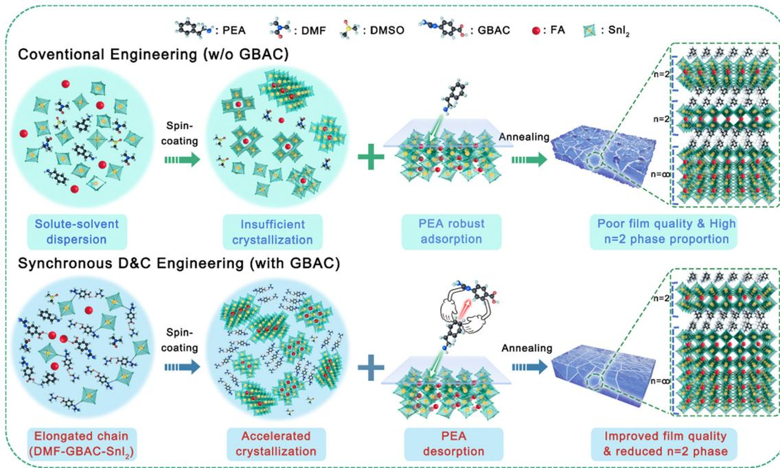
Scheme 1 Schematic illustration of synchronous dimension-crystallization (D&C) engineering.
