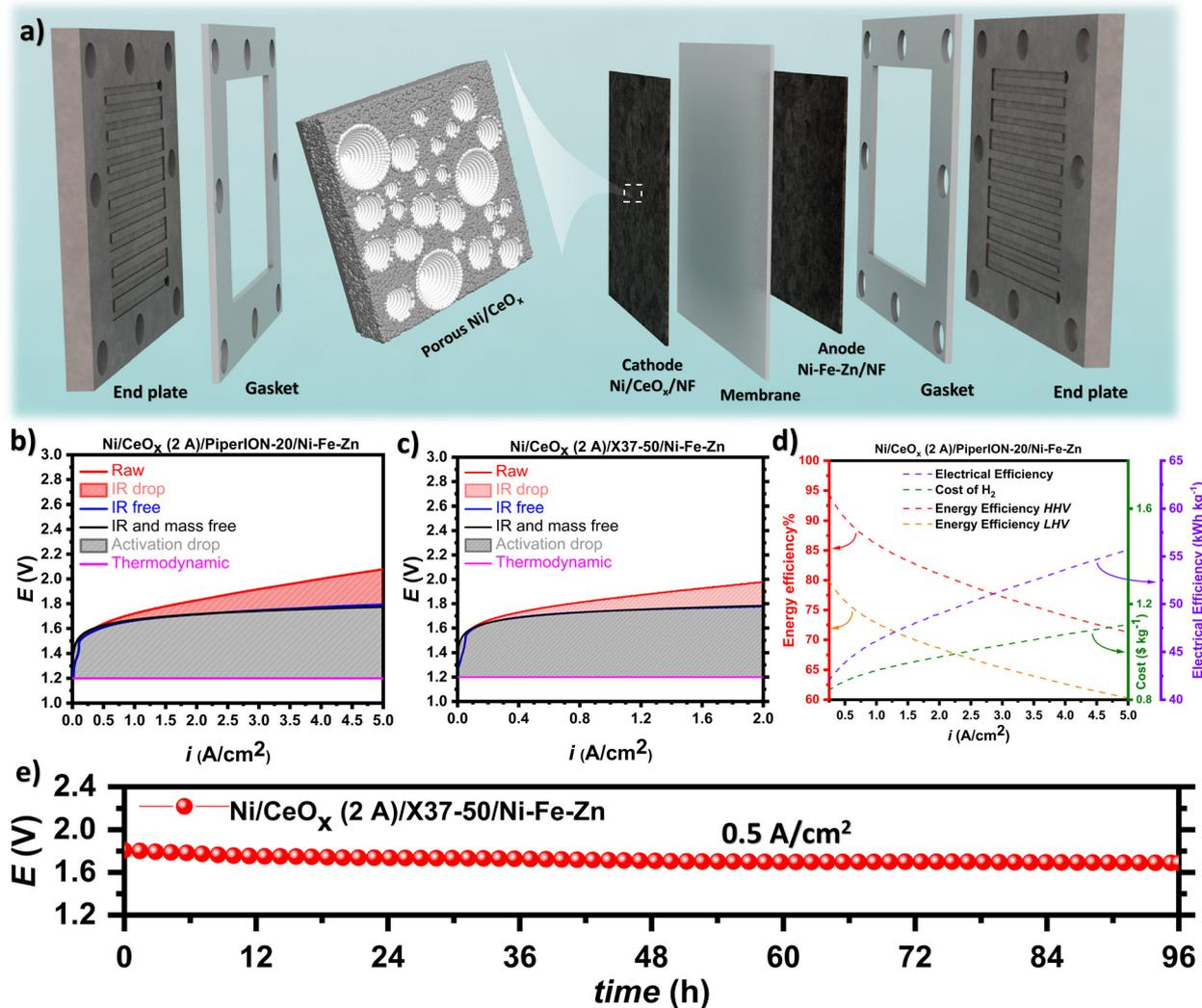
Fig. 4 AEMWE measurements. (a) Schematic diagram of an AEMWE. Deconvoluted LSV at 60 °C for (b) AEMWE with PiperION-20 and (c) AEMWE with X37-50. (d) Energy and electrical efficiencies of AEMWE with PiperION-20 at 60 °C. (e) Chronopotentiogram at 0.5 A cm<sup>-2</sup> for the AEMWE with X37-50 at 60 °C.
