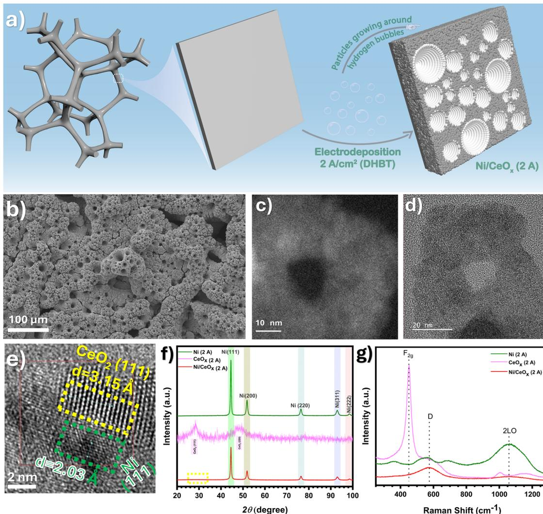
Fig. 1 Synthesis, morphology, and structure. (a) A schematic representation of the synthesis of Ni/CeO<sub>x</sub> (2 A). (b) SEM, (c) dark-field STEM, (d) and (e) HR-TEM images of Ni/CeO<sub>x</sub> (2 A). (f) XRD patterns and (g) Raman spectra of the designed films.
