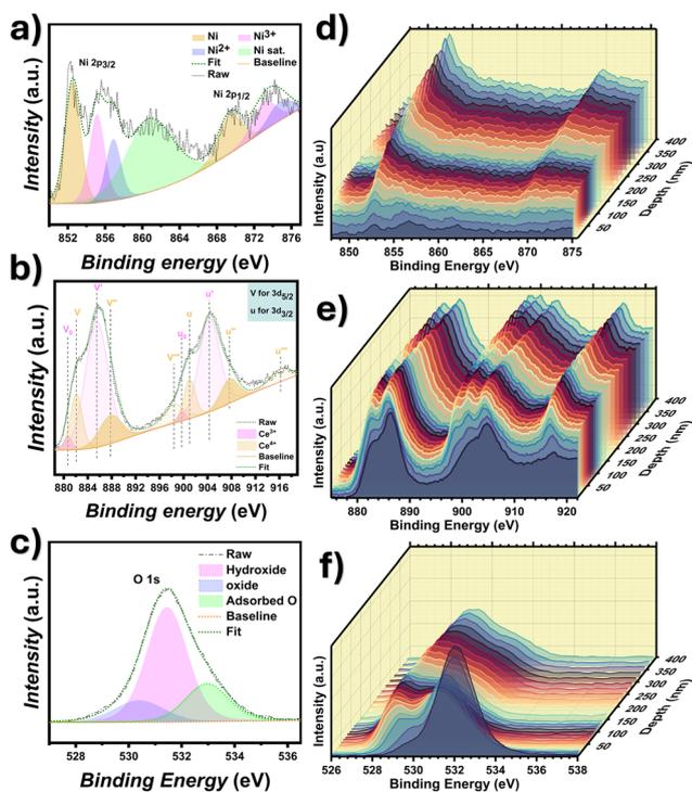
Fig. 2 XPS spectra of the Ni/CeO<sub>x</sub> (2 Å) catalyst. Top-surface (a)–(c) and depth-profiling (d)–(f) XPS spectra of the Ni/CeO<sub>x</sub> (2 Å) film. Ni 2p spectra (a) and (d), Ce 3d spectra (b) and (e), and O 1s spectra (c) and (f).
