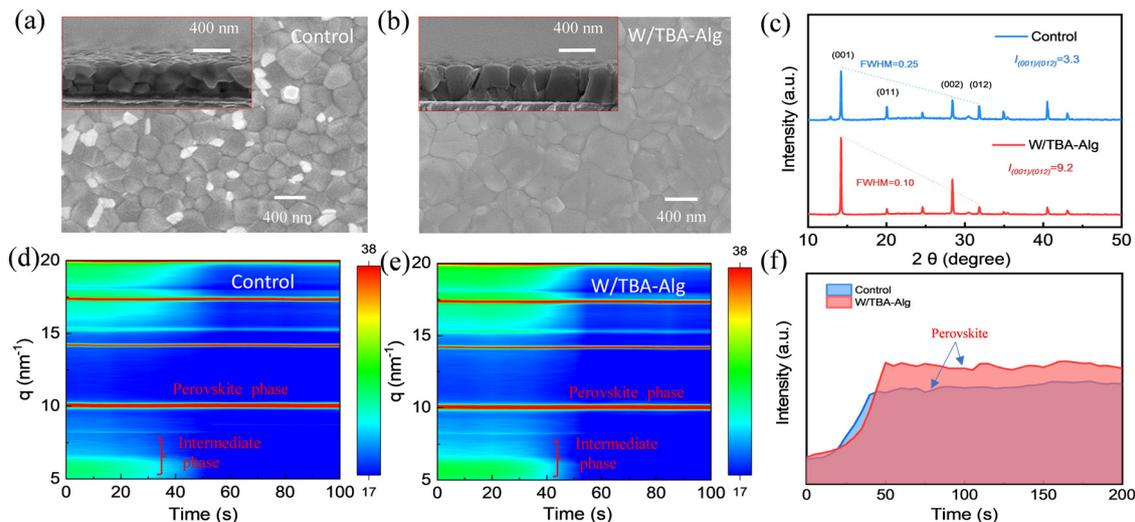
Fig. 2 Top-view and cross-sectional SEM images of (a) the control film and (b) the film with TBA-Alg treatment. (c) XRD patterns of the control and TBA-Alg-treated perovskite films. Temporal evolution of *in situ* GIWAXS patterns during annealing (d) control and (e) TBA-Alg-treated perovskite films. (f) Time-resolved integrated peak area intensity for black phases of the control and the TBA-Alg-treated perovskites ( $q = 9.98 \text{ nm}^{-1}$ ).
