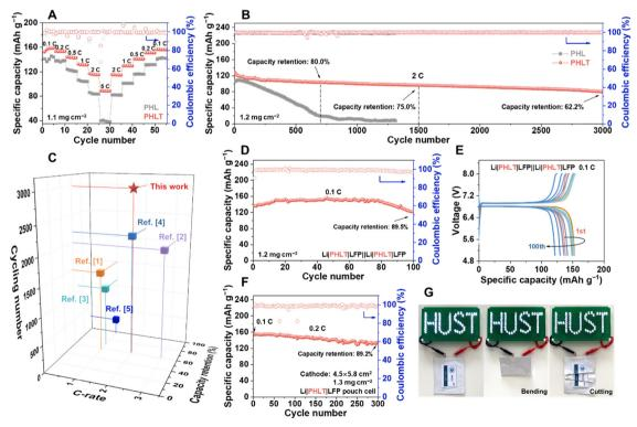
Fig. 6 (A) Rate capabilities and (B) cycling stability of the Li||LFP cells. (C) A comparison of C-rate, cycling number, and capacity retention between this work and other reported PVDF-based electrolytes in recent literature. (D) Cycling stability and (E) charge/discharge voltage profiles of the bipolar stacking cell. (F) The cycling performance of a Li|PHLT|LFP pouch cell at 0.2 C. (G) Optical photographs illustrating the bending and cutting tests of the pouch cell
