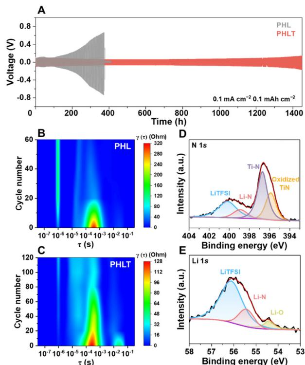
Fig. 4 (A) Lithium stripping-plating profiles at  $0.1 \text{ mA cm}^{-2}$  and  $0.1 \text{ mA h cm}^{-2}$ . DRT results of the (B) Li|PHL|Li and (C) Li|PHLT|Li cells cycled at  $0.2 \text{ mA cm}^{-2}$  and  $0.2 \text{ mA h cm}^{-2}$ . *Ex situ* XPS analysis of (D) N 1s and (E) Li 1s spectra of recovered TiN nanofibers.
