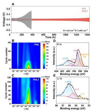
Fig. 4 (A) Lithium stripping-plating profiles at  $0.1 \, \text{mA cm}^{-2}$  and  $0.1 \, \text{mA h cm}^{-2}$ . DRT results of the (B) Li|PHL|Li and (C) Li|PHLT|Li cells cycled at 0.2 mA  $\rm cm^{-2}$ and 0.2 mA h cm<sup>-2</sup>. Ex situ XPS analysis of (D) N 1s and (E) Li 1s spectra of recovered TiN nanofibers.
