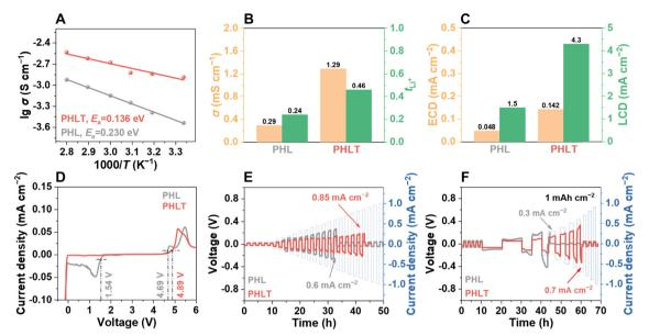
Fig. 3 (A) Arrhenius plots of the QPEs. (B) Ionic conductivity and Li<sup>+</sup> transference number, (C) exchange current density (ECD) and limiting current density (LCD) results, (D) LSV curves and CCD tests using (E) time-constant mode (1 h for platting and 1 h for stripping), and (F) the capacity-constant mode (1 mA h cm<sup>-2</sup>) at 25 °C, respectively.
