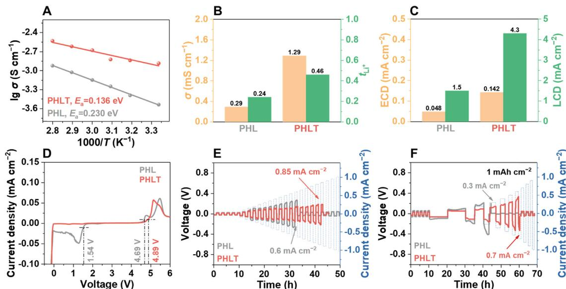
Fig. 3 (A) Arrhenius plots of the QPEs. (B) Ionic conductivity and  $\text{Li}^+$  transference number, (C) exchange current density (ECD) and limiting current density (LCD) results, (D) LSV curves and CCD tests using (E) time-constant mode (1 h for plating and 1 h for stripping), and (F) the capacity-constant mode ( $1 \text{ mA h cm}^{-2}$ ) at  $25^\circ\text{C}$ , respectively.
