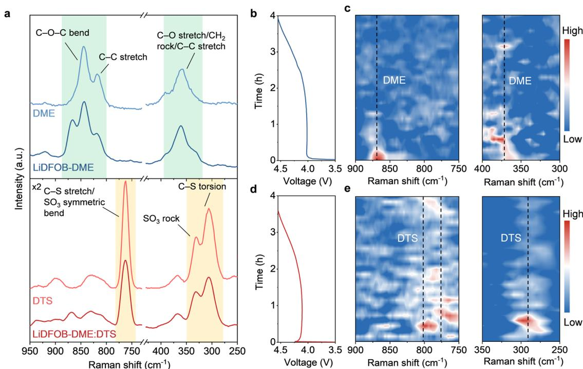
Fig. 2 Electric double layer (EDL) structure evolution during the charging process. (a) Raman spectra of different electrolytes and the corresponding pure solvent. Voltage *versus* time profiles and *in situ* Raman spectra near the interface of the LiCoO<sub>2</sub> electrode during the charging process in (b) and (c) LiDFOB–DME and (d) and (e) LiDFOB–DME:DTS electrolytes.
