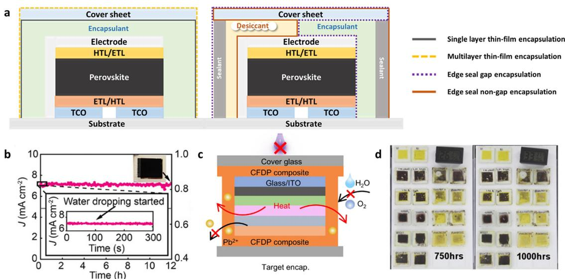
**Fig. 17** (a) Schematic diagrams of different TFE and ES encapsulation approaches. (b) High stability performance under water drop stress.<sup>136</sup> (c) Schematic of CFDP package without UV irradiation.<sup>257</sup> (d) The degradation performance after 750 and 1000 hours.<sup>258</sup> Copyright 2016, Elsevier Ltd.
