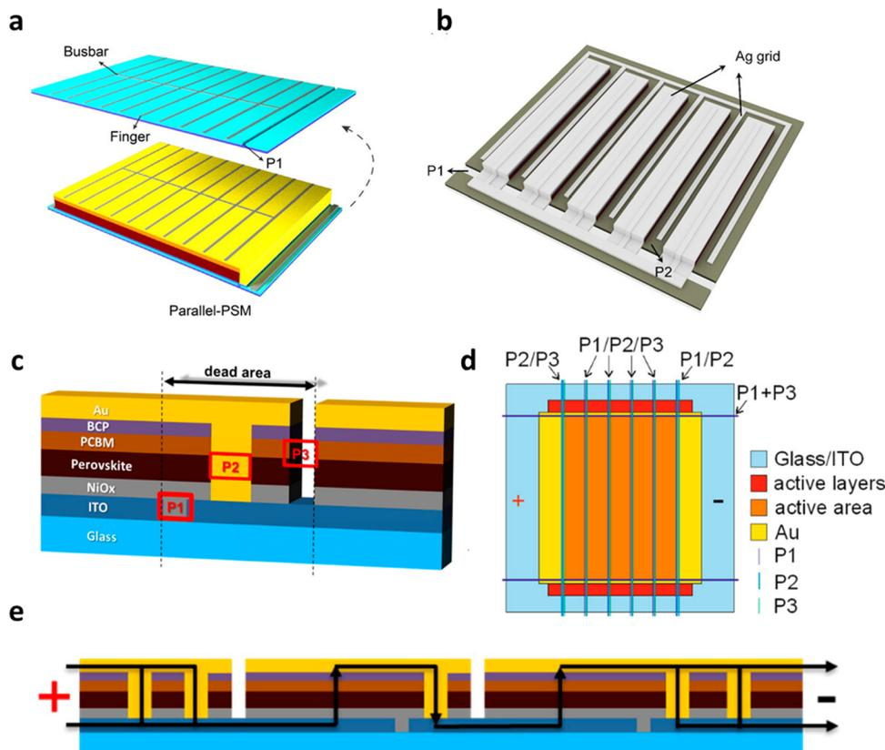
Fig. 1 (a) Architecture of the parallel PSMs.<sup>40</sup> Copyright 2021, Wiley-VCH GmbH. (b) Metallic grids on parallel PSMs.<sup>43</sup> Copyright 2021, American Association for the Advancement of Science. (c) P1–P2–P3 laser scribing on series PSMs. (d) The overall plane view and (e) the current flow path in the side view of the series PSMs.<sup>44</sup> Copyright 2020, MDPI, Basel, Switzerland.
