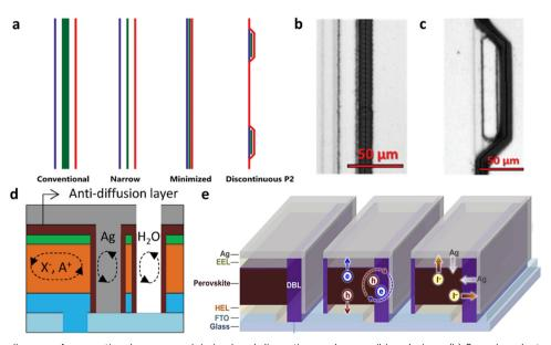
Fig. 3 (a) Schematic diagram of conventional, narrow, minimized and discontinuous laser scribing designs. (b) Scanning electron microscope (SEM) figures of minimized and (c) discontinuous P2 interconnection. 60 Copyright 2024, Wiley-VCH GmbH. (d) Anti-diffusion layer treated by O<sub>3</sub>. 61 Copyright 2023, Wiley-VCH GmbH. (e) DBL for blocking lateral diffusion.<sup>62</sup> Copyright 2019, Elsevier Inc.
