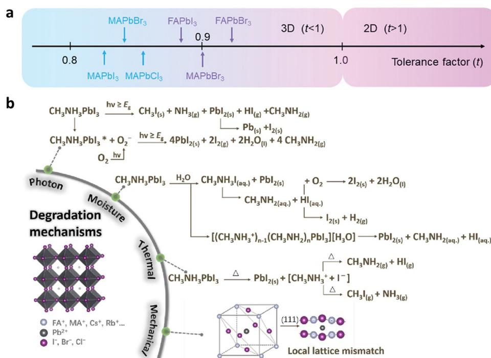
Fig. 16 (a) Tolerance factors distribution of different perovskite compositions.<sup>233</sup> Copyright 2022, Wiley-VCH GmbH (b) The instability stress sources of perovskite materials.<sup>234</sup>
