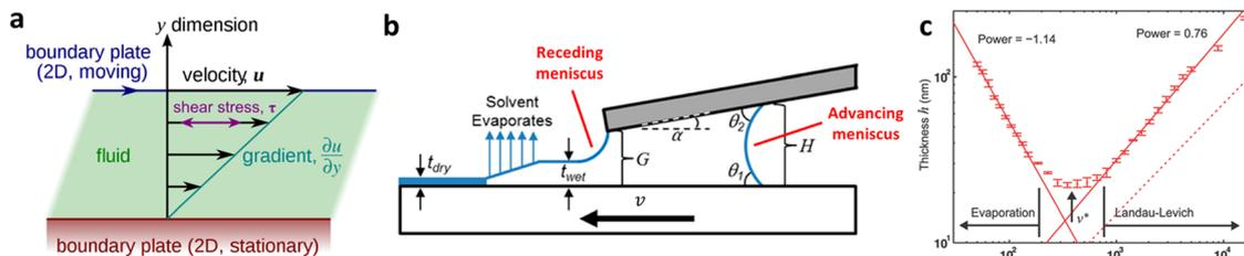
Fig. 5 (a) Schematic diagram of fluid dynamics of the meniscus coating process. (b) Schematics of the functions relationships between speed and perovskite thickness under evaporation and Landau–Levich regimes.<sup>80</sup> (c) Measured film thickness  $h$  as a function of deposition speed  $v$ .<sup>79</sup> Copyright 2009, American Chemical Society.
