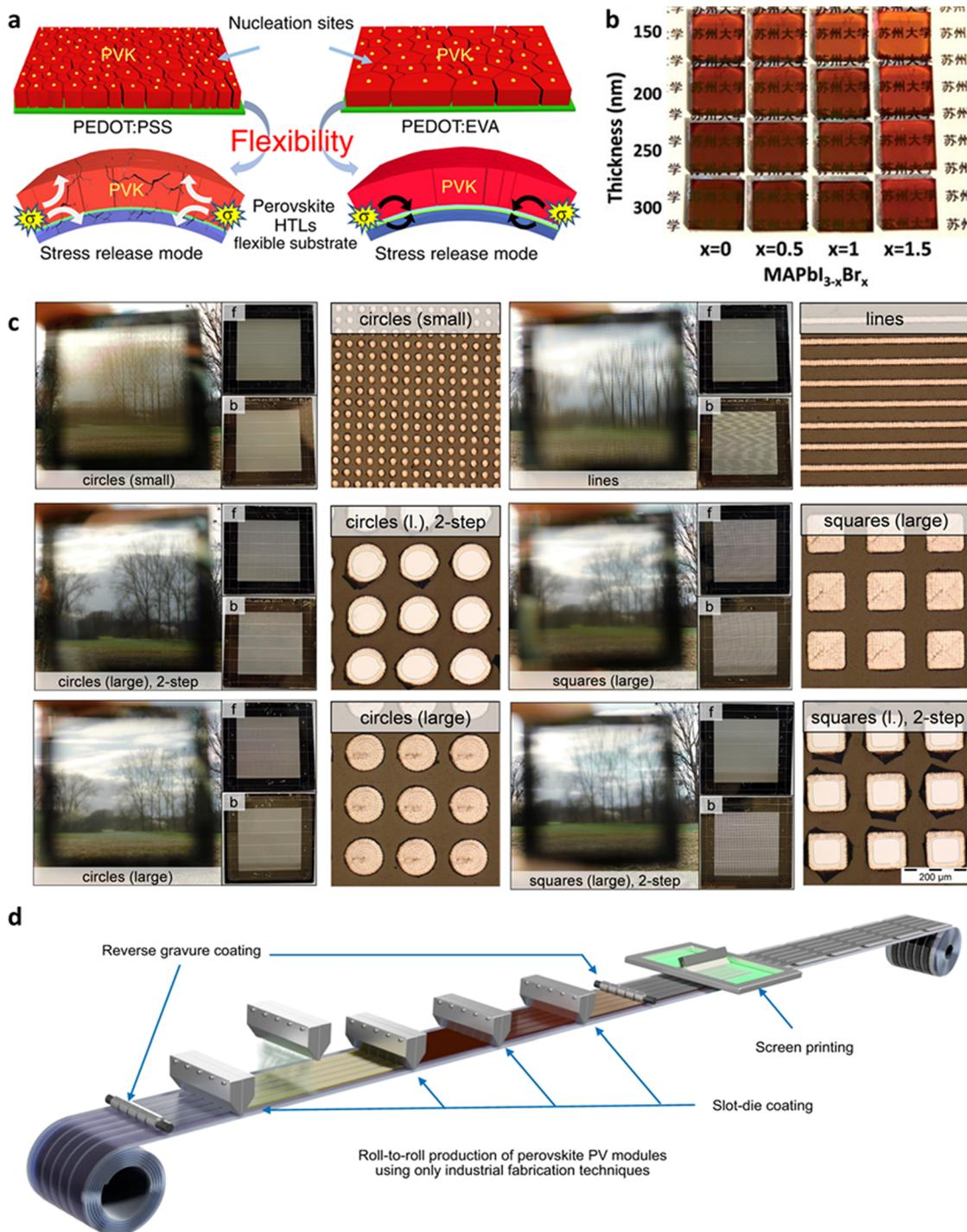
Fig. 4 (a) Schematic diagram of PEDOT:EVA stress relief.<sup>67</sup> (b) Transmittance changes with the amount of Br and the perovskite thickness.<sup>68</sup> (c) Transparency effect under different laser patterns.<sup>69</sup> (d) Schematic diagram of the large-scale R2R PSMs production process with the help of multi-process collaboration.<sup>70</sup>
