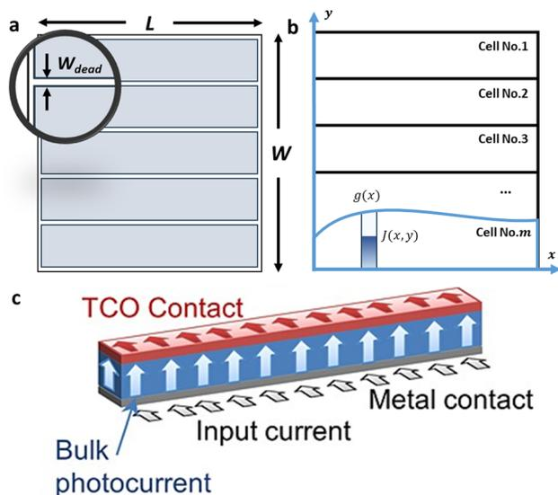
Fig. 2 (a) Schematic diagram of subcells distribution segment. (b) Current flow in one arbitrarily segment.<sup>50</sup> (c) Schematic of the vertical current flow received from the back bottom and collected from the edge of the TCO contact in subcells.<sup>51</sup> Copyright 2013, John Wiley & Sons, Ltd.
