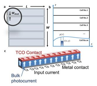
**Fig. 2** (a) Schematic diagram of subcells distribution segment. (b) Current flow in one arbitrarily segment. (c) Schematic of the vertical current flow received from the back bottom and collected from the edge of the TCO contact in subcells.  $^{51}$  Copyright 2013, John Wiley & Sons, Ltd.
