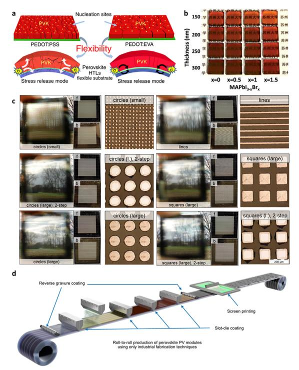
Fig. 4 (a) Schematic diagram of PEDOT:EVA stress relief.<sup>67</sup> (b) Transmittance changes with the amount of Br and the perovskite thickness.<sup>68</sup> (c) Transparency effect under different laser patterns. <sup>69</sup> (d) Schematic diagram of the large-scale R2R PSMs production process with the help of multiprocess collaboration.<sup>70</sup>
