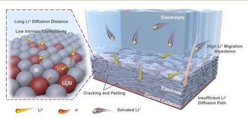
Fig. 1 Limiting factors causing poor kinetic performances of Si anodes at particle, interface, and electrode levels.
