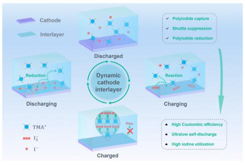
Fig. 1 Schematic of the evolution of the dynamic cathode interlayer in the Zn-I<sub>2</sub> battery.
