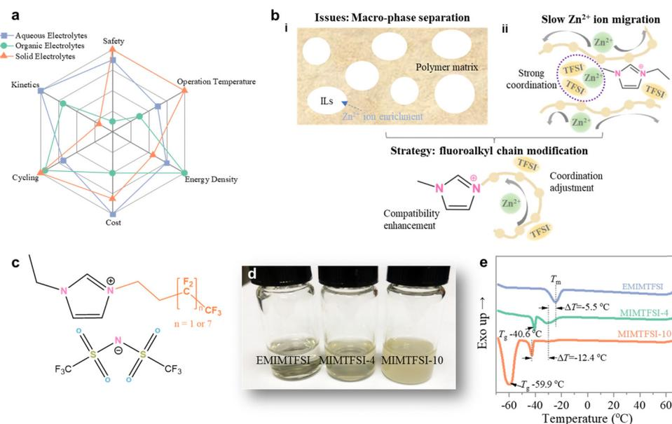
**Fig. 1** Design strategy and characteristics of F-IL plasticizers. (a) Comparison of various electrolytes for ZIBs; (b) illustration of the accelerated ion conduction by F-IL plasticizers, where F-ILs not only enhance the compatibility with the polymer matrix but also improve the Zn<sup>2+</sup> ion solvation structure; (c) chemical structures of as-synthesized F-ILs; (d) optical pictures of the ILs; (e) DSC test of the ILs.
