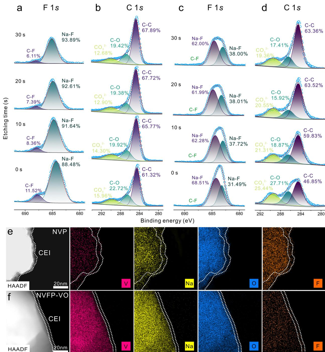
Fig. 5 *Ex situ* characterizations of NVP and NVFP-VO cathodes. In-depth element distributions and high-resolution XPS spectra of F 1s and C 1s. (a) and (b) NVP, and (c) and (d) NVFP-VO. HAADF-STEM and STEM-EDS mappings of (e) NVP and (f) NVFP-VO.
