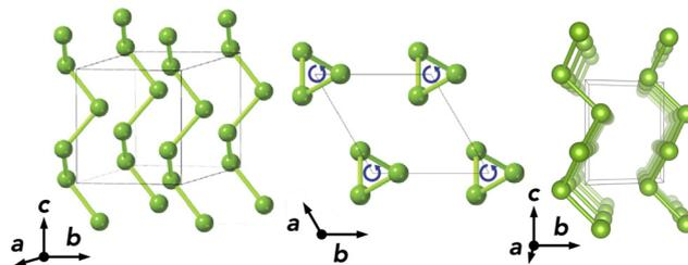
Fig. 1 Crystal structure of trigonal selenium (t-Se) along various lattice directions. Adapted with permission from Kumagai *et al.*<sup>3</sup>
