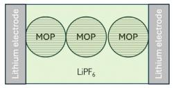
Fig. 15 Wet case conductivity. Electron transfer reactions occur at the lithium electrode/MOP interface, where lithium transfer reactions occur both at the lithium electrode/MOP and lithium electrode/electrolyte interfaces
