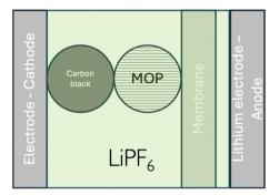
Fig. 9 Schematic illustration of a LiMO<sub>2</sub> lithium battery
