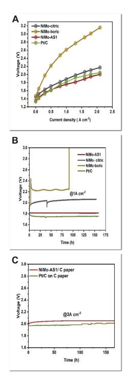
Fig. 3 (A) Polarization curves of AEMWEs with NiMo-AS1, NiMo-citric, and NiMo-boric on C paper as the cathode, respectively; (B) long-term electrolysis data at a constant current density of 1 A cm $^{-2}$  and cell temperature of 80  $^{\circ}$ C; (C) electrolysis at a current density of 3 A cm<sup>-2</sup> at 80 °C.
