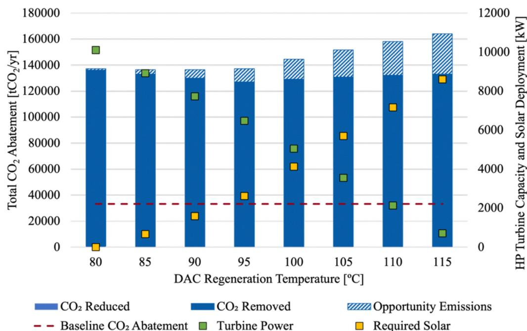
Fig. 15 CO<sub>2</sub> abatement potential for DAC in series – downstream of the HP ORC configuration. Note the reinjection temperature is synonymous with the DAC regeneration temperature in this configuration.
