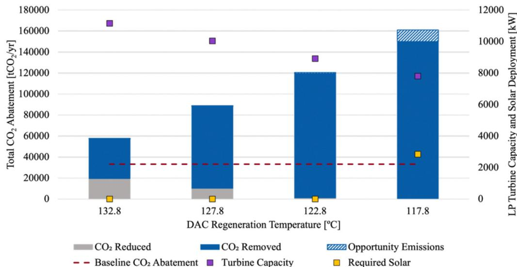
Fig. 14 CO<sub>2</sub> abatement potential for DAC in series – upstream of the LP ORC configuration, exhibiting the turbine power and solar deployment required to meet the DAC electricity needs in each test case. Various regeneration temperatures were tested, all within 20 °C of the production well temperature.
