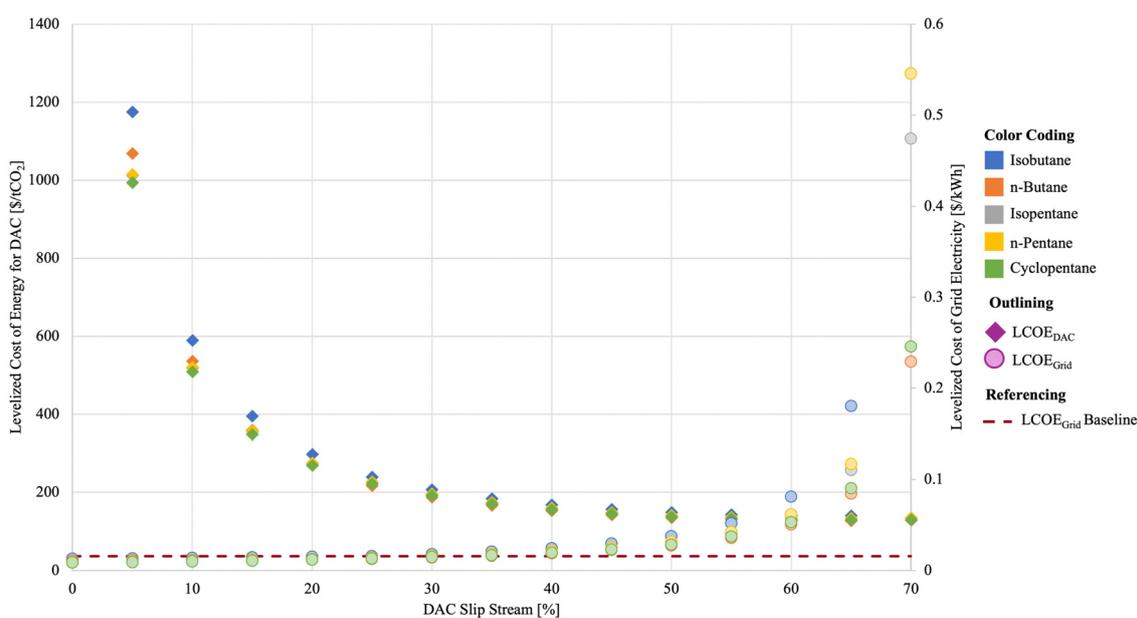
**Fig. 10** Technoeconomic results for DAC in parallel configuration using a high-temperature geothermal reservoir, illustrating the levelized cost of energy delivered to DAC (LCOE<sub>DAC</sub>), levelized cost of grid electricity generation (LCOE<sub>Grid</sub>), and the LCOE<sub>Grid</sub> baseline value, for all working fluids evaluated.
