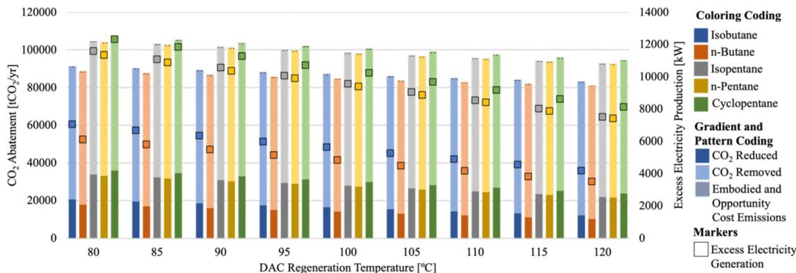
**Fig. 11** CO<sub>2</sub> abated for the DAC in series – downstream configuration for a geothermal reservoir temperature of 225 °C, showing grid electricity generation using a variety of working fluids: isobutane (blue gradient), *n*-butane (orange gradient), isopentane (gray gradient), *n*-pentane (yellow gradient), and cyclopentane (green gradient).
