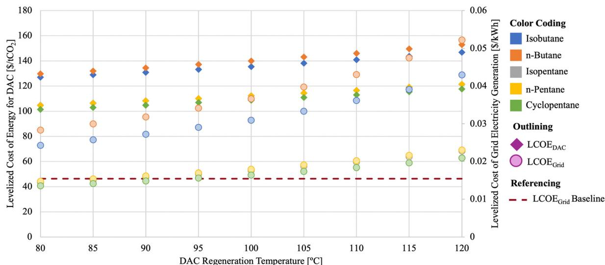
Fig. 12 Technoeconomic results from evaluating DAC in series – downstream with a high-temperature geothermal reservoir, illustrating the levelized cost of energy delivered to the DAC system ( $\text{LCOE}_{\text{DAC}}$ ) and levelized cost of grid electricity generation ( $\text{LCOE}_{\text{Grid}}$ ), compared to the levelized cost of grid electricity from the binary geothermal power plant baseline ( $\text{LCOE}_{\text{Grid}}$  baseline).
