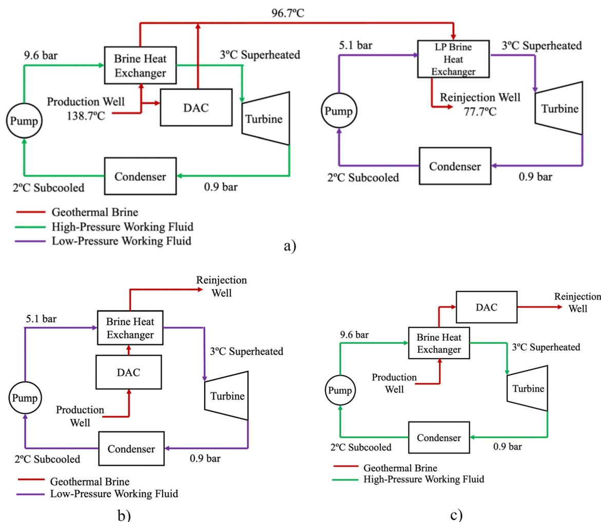
**Fig. 5** Configurations evaluated throughout the geothermal-DAC integration study. Each can be referred to (a) DAC in parallel with combined cycle power plant, (b) DAC in series – upstream of the LP ORC, and (c) DAC in series – downstream of the HP ORC, each referring to the position of the DAC regeneration system.
