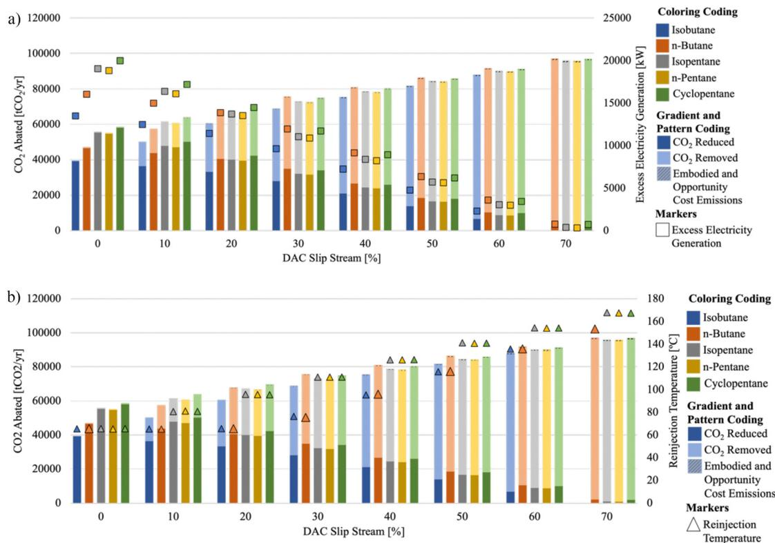
**Fig. 9** CO<sub>2</sub> abated in the DAC in parallel configuration for a geothermal reservoir temperature of 225 °C, showing (a) grid electricity generation, and (b) reinjection well temperature, using a variety of working fluids: isobutane (blue gradient), *n*-butane (orange gradient), isopentane (gray gradient), *n*-pentane (yellow gradient), and cyclopentane (green gradient).
