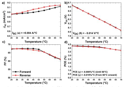
Fig. 2 Effect of temperature on the key photoelectrical parameters (a) temperature dependence of  $V_{SC}$ , (b) temperature dependence of  $V_{CC}$ , (c) temperature dependence of FF, and (d) temperature dependence of PCE) of the OPV module over a temperature range of 25-70 °C under AM1.5G conditions during upward (black) and downward (red) direction.
