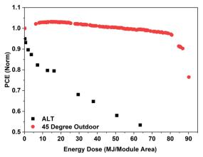
Fig. 5 PCE values, normalized to  $t_0$  performance, as a function of light energy dose incident onto the module surface in megajoules (MJ) during accelerated lifetime testing (black points) and during the one-year outdoor exposure at a 45° inclination angle (red points).
