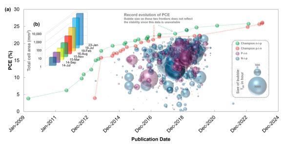
Fig. 3 Chronological evolution of perovskite solar cells. (a) power conversion efficiency (PCE) and  $T_{80}$  lifetime of perovskite solar cells in bubble chart.<sup>33</sup> (b) total cell area of annual champion perovskite solar cells.<sup>33</sup>  $T_{80}$  refers to the time at which the performance of a perovskite solar cell attains 80% of its initial value in ambient conditions.
