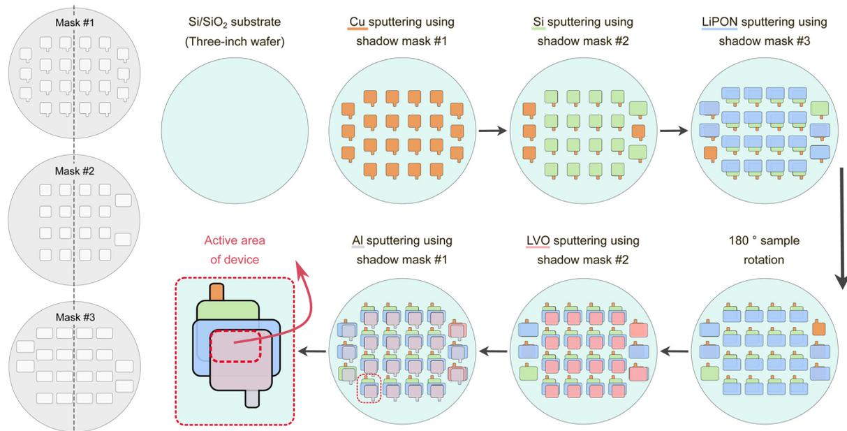
**Fig. 1** Illustration of shadow masks used for *in situ* patterning of devices and their fabrication sequence. In this case, 16 SSBs and diagnostic devices were fabricated simultaneously in a 3-inch silicon wafer. Materials used: copper as anode current collector, amorphous silicon (a-Si) as anode, lithium phosphorus oxynitride (LiPON) as electrolyte, lithium vanadium oxide (LVO) as cathode, and aluminum as cathode current collector.
