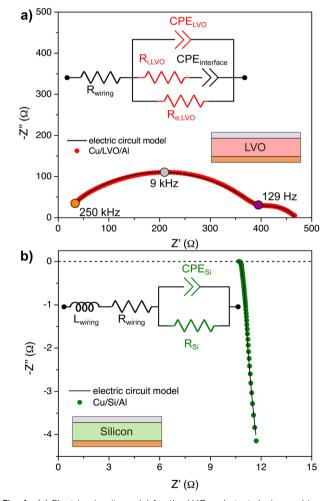
Fig. 4 (a) Electric circuit model for the LVO-only test device and impedance spectrum at OCV. (b) Impedance spectrum of Si-only diagnostic device at OCV and the electric circuit model that represents this device.
