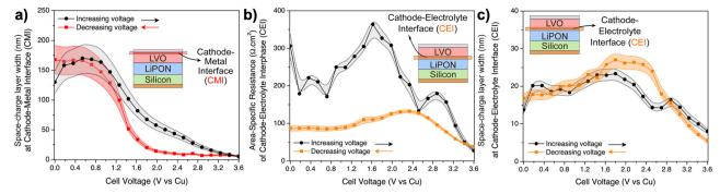
Fig. 9 Interfacial properties of the thin-film SSB computed from the circuit parameters as a function of applied cell voltage. (a) Space-charge layer (SCL) at the LVO-Al interface; (b) resistance of LVO-LiPON interphase; (c) SCL at the LVO-LiPON interphase
