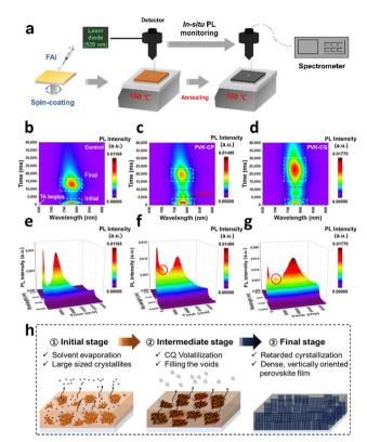
Fig. 5 In situ PL measurements during the FA-based PVK crystallization. (a) Schematic illustration of in situ PL monitoring during the FA-based PVK crystallization (150 °C). Heatmaps of in situ PL of the FA-based PVK film for (b) control, (c) PVK-CP, and (d) PVK-CQ. 3D colormap surfaces of in situ PL of the FA-based PVK film for (e) control, (f) PVK-CP, and (g) PVK-CQ. (h) Schematic summary showing the effects of CQ in crystallization kinetics.
