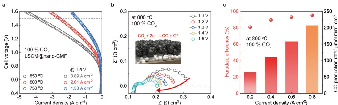
Fig. 5 Extremely high- $\text{CO}_2$  electrolysis performance of SOEC: (a)  $I$ - $V$  curves of  $\text{CO}_2$  electrolysis using the LSCM@nano-CMF electrode under pure  $\text{CO}_2$ . (b) EIS data of LSCM@nano-CMF fuel electrode at  $800\text{ }^\circ\text{C}$  under bias conditions. (c) Faradaic efficiency of  $\text{CO}_2$  electrolysis using LSCM@nano-CMF fuel electrode at  $800\text{ }^\circ\text{C}$  under pure  $\text{CO}_2$ .
