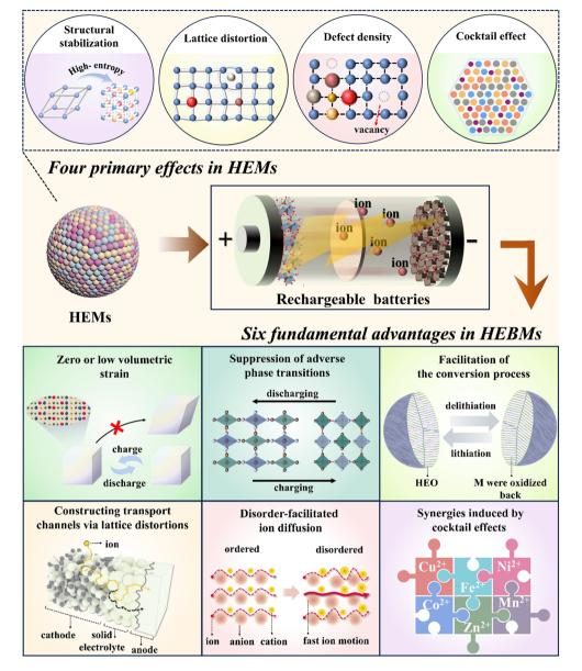
Fig. 2 Fundamental advantages of HEMs in battery materials design.
