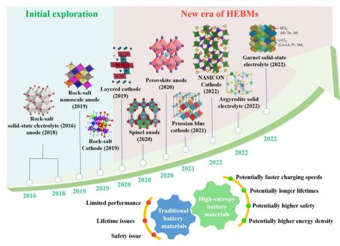
Fig. 1 The historical development of HEBMs with different structural characteristics, including rock-salt, layered, spinel, perovskite, PBA, NASICON, garnet, and argyrodite phases.
