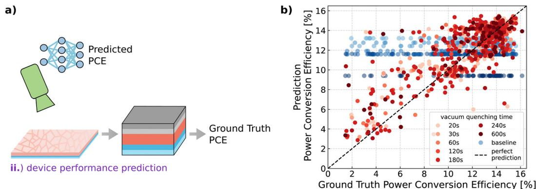
**Fig. 3** Device performance prediction. (a) Extension of the predictive approach from the material to the device level by predicting device performance even before perovskite thin films are completed into solar cells. (b) Predicting holistic device performance through deep-learning-augmented evaluation of *in situ* monitoring data provides early in-line assessments of perovskite thin-film quality.
