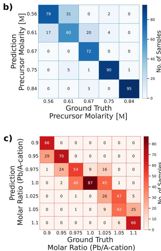
Fig. 2 Material composition monitoring. (a) Variations in precursor molarity and the molar ratio are detected through *in situ* metrology augmented by deep learning. (b) and (c) Deep neural networks learn to classify variations in precursor molarity (b) and molar ratio (c). This capability enables *in situ* detection of deviations from the targeted material composition.
