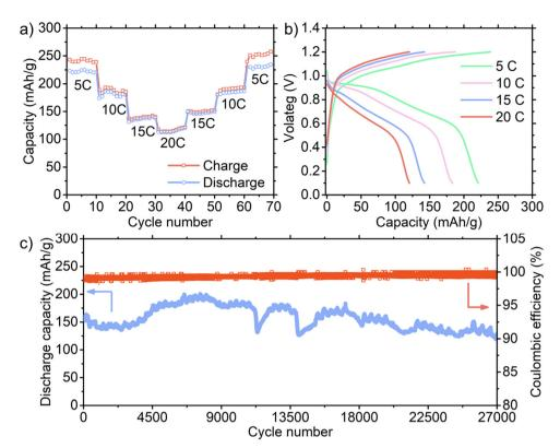
Fig. 4 (a) Specific capacity and of the full cell with 8% active material loading of PANI-sandwiched CNT cathode at different C rates (1C = 300 mA per g). (b) Corresponding charge/discharge voltage profiles at different C rates. (c) Specific discharge capacity and Coulombic efficiency as a function of cycle number at 15C for 8 wt% active material loading cell.
