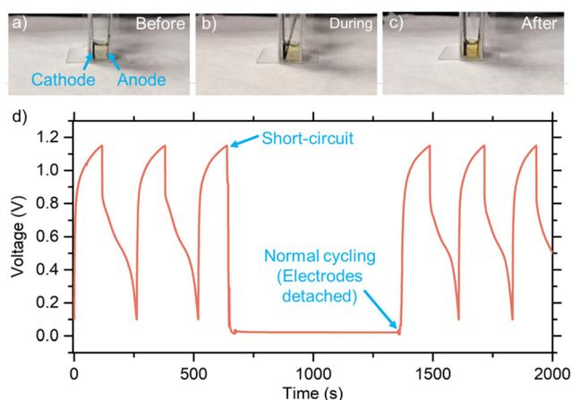
Fig. 6 Test setup with a cathode and an anode in the electrolyte ( $\sim 590 \mu\text{L}$ ) with three different electrode configurations (a) before, (b) during, and (c) after the short circuit, and (d) corresponding voltage profile against time.
