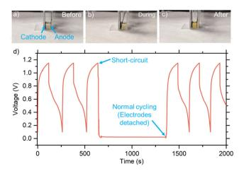
Fig. 6 Test setup with a cathode and an anode in the electrolyte  $(\sim 590 \mu L)$  with three different electrode configurations (a) before, (b) during, and (c) after the short circuit, and (d) corresponding voltage profile against time
