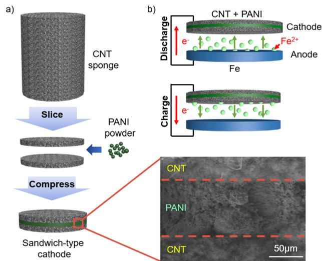
**Fig. 1** (a) Fabrication of the cathode by slicing cylindrical sponge-like CNT and then sandwiching PANI powder. The SEM image shows a PANI-impregnated layer between the CNT layers. (b) Illustration of discharging and charging processes and corresponding flow of Fe ions and electrons.
