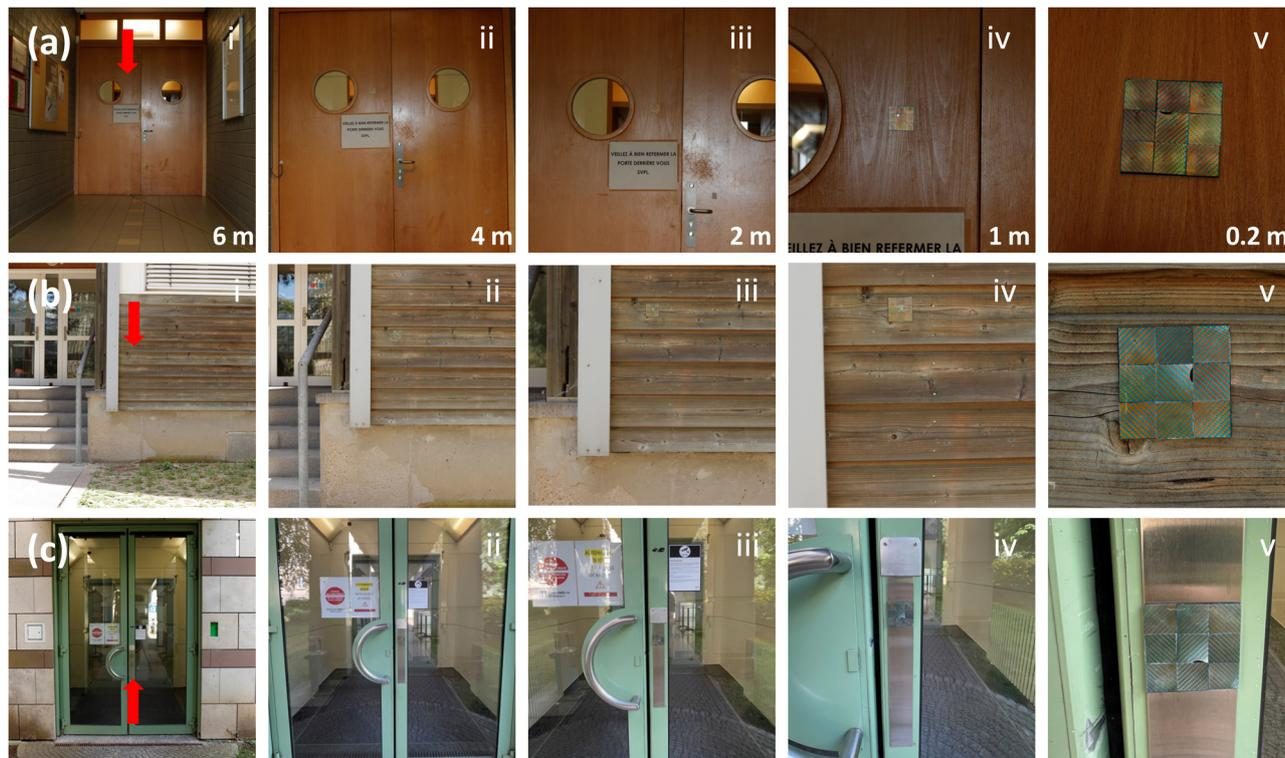
Fig. 4 Photographs of a 7.5 cm by 7.5 cm array of RGB-pixelated polymerised CLC film placed on a wooden door and illuminated by indoor diffuse ambient light (top row), an outdoor wooden wall illuminated by indirect sunlight on a sunny day (middle row) and a silver-coloured metal panel on a door outside, also illuminated by indirect sunlight on a sunny day. For each situation, panels i to v are obtained with stepwise reduced photography distance, as indicated in the top row.
