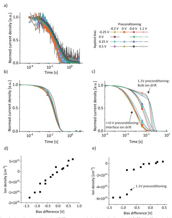
Fig. 4 (a) Normalized experimental and (b) simulated BACE measurements in the high ion density regime. (c) BACE drift-diffusion simulations with a 2 orders of magnitude lower ion density (10<sup>15</sup> cm<sup>-3</sup>). (d) and (e) Ion density resulting from the integrated BACE current density simulations for the high and low ion density regime, respectively.
