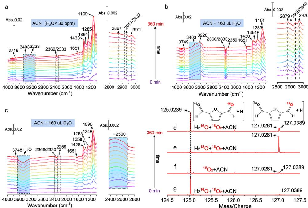
Fig. 5 *In situ* ATR-SEIRAS measurement of HMF selective to DFF over Cd<sub>0.75</sub>Zn<sub>0.25</sub>S in different reaction mediums: (a) ACN; (b) ACN + H<sub>2</sub>O; and (c) ACN + D<sub>2</sub>O. (d)–(g) High-resolution mass spectrum of the products using different isotopes.
