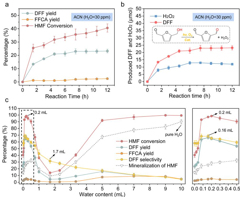
Fig. 1 (a) Time-dependent HMF conversion, DFF yield and FFCA yield in ACN over Cd<sub>0.75</sub>Zn<sub>0.25</sub>S. (b) Time-dependent DFF and H<sub>2</sub>O<sub>2</sub> production in ACN over Cd<sub>0.75</sub>Zn<sub>0.25</sub>S. (c) HMF oxidation activity of Cd<sub>0.75</sub>Zn<sub>0.25</sub>S in a mixed solution of ACN and H<sub>2</sub>O (V<sub>H<sub>2</sub>O</sub> + V<sub>ACN</sub> = 10 mL; reaction time: 12 h).
