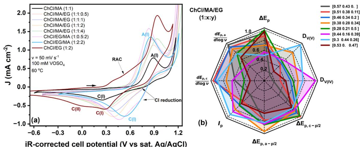
Fig. 4 Electrochemical analysis of ternary mixtures based on ChCl/MA and EG. (a) CVs highlighting the parent DES and the ternary mixture with the most reversible kinetics at 60 °C and 50 mV s<sup>-1</sup>: ChCl/EG/MA (1:2:2). (b) Radar plot of electrochemical metrics extracted from CVs across the ternary mixtures expressed as mass fractions.
