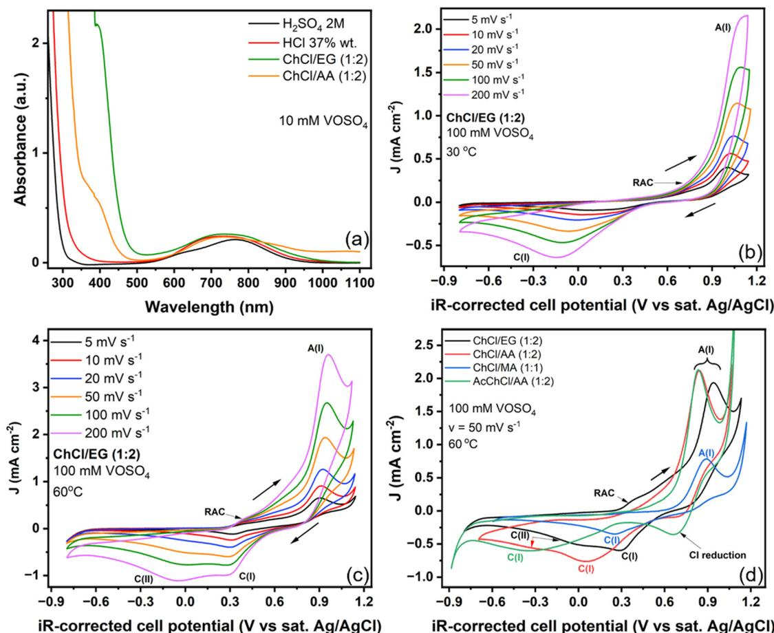
**Fig. 2** (a) Spectroscopic characterization of VOSO<sub>4</sub> in type III DES: UV-vis spectra of VOSO<sub>4</sub> in DES and aqueous solutions. (b) CVs of VOSO<sub>4</sub> in ChCl/EG (1 : 2) at 30 °C. (c) CVs of VOSO<sub>4</sub> in ChCl/EG (1 : 2) at 60 °C. (d) Comparison of voltammograms from VOSO<sub>4</sub> in the studied DES at 60 °C and a scan rate of 50 mV s<sup>-1</sup>.
