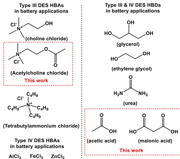
Fig. 1 Type III & IV DES applied to batteries.
