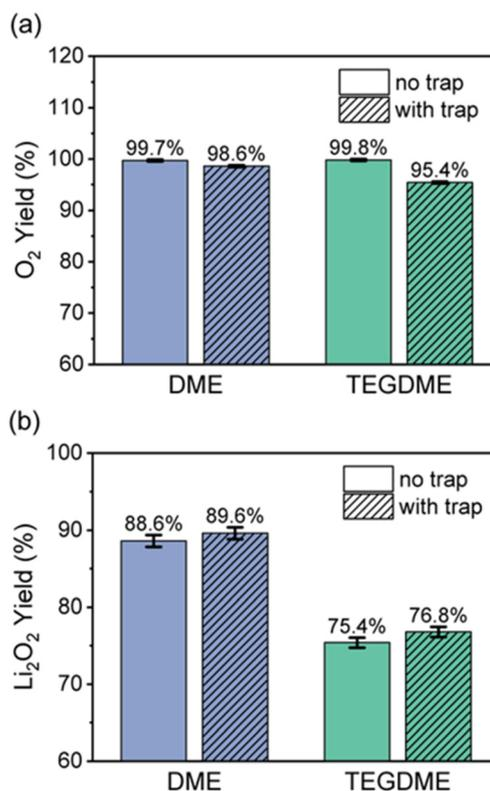
**Fig. 1** (a) Oxygen and (b)  $\text{Li}_2\text{O}_2$  yields after  $\text{KO}_2$  disproportionation in DME (blue) and TEGDME (green) without and with singlet oxygen trap, showing no evidence of  $^1\text{O}_2$  or  $\text{O}_2^-$  reactivity.
