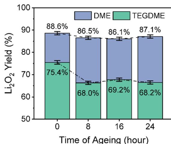
**Fig. 3** Quantity of  $\text{Li}_2\text{O}_2$  as a percentage of the theoretical yield of  $\text{Li}_2\text{O}_2$  after the  $\text{KO}_2$  disproportionation reaction, in DME (blue) and TEGDME (green), has gone to completion. The quantity of  $\text{Li}_2\text{O}_2$  was determined immediately after the reaction was complete (0 hours), and after a further 8, 16 and 24 hours of ageing.
