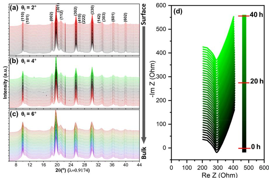
**Fig. 6** Grazing-incidence XRD patterns of LYC\_PMMA pellets as a function of air exposure time, collected at an incidence beam angle of (a) 2°, (b) 4°, and (c) 6° ( $2\theta$ ), respectively. The patterns were collected every 6 min within a total exposure time of 150 min. (d) *Operando* time-resolved EIS spectra of a symmetric SS|LYC\_PMMA|SS cell recorded as a function of air exposure time to evaluate the air stability of LYC\_PMMA SE.
