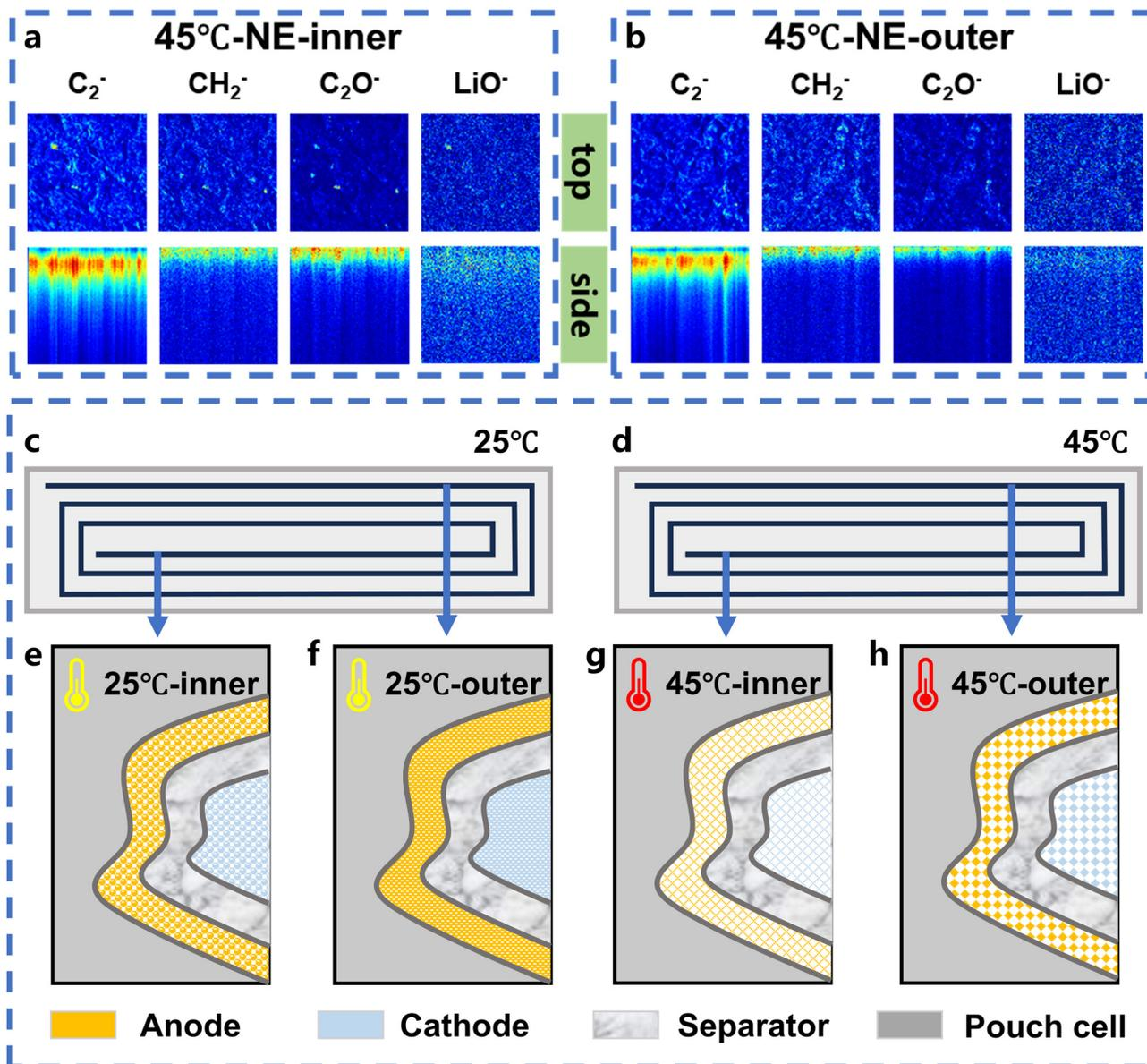
**Fig. 6** TOF-SIMS chemical maps of various secondary ion fragments at 45 °C: (a) inner anode and (b) outer anode. Cross-sectional schematic of a pouch cell (c) at 25 °C and (d) 45 °C. (e–h) Schematic diagram of inner and outer cell structure at 25 °C and 45 °C.
