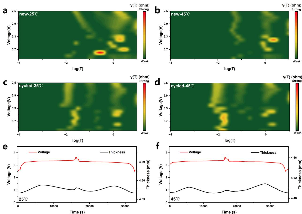
Fig. 2 DRT patterns of fresh batteries (a) at 25 °C and (b) at 45 °C. DRT patterns of cycled batteries (c) at 25 °C and (d) at 45 °C. *In situ* mechanical testing of phase transition and expansion changes: *in situ* expansion analysis for (e) at 25 °C and (f) at 45 °C.
