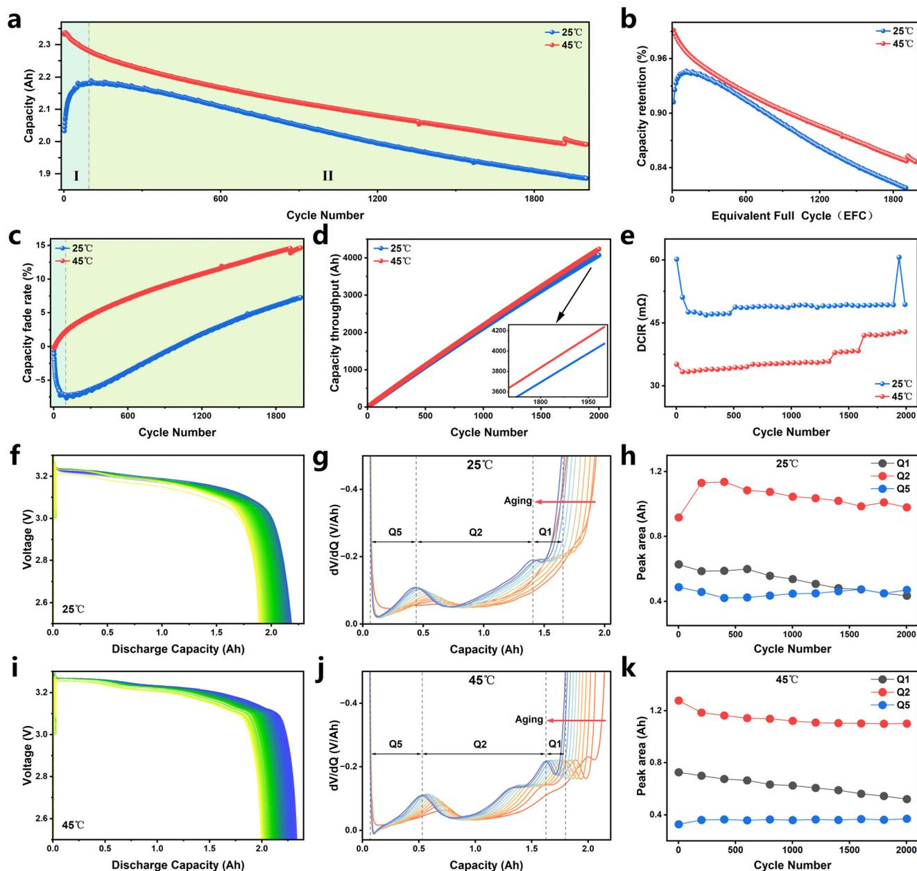
**Fig. 1** Comparison of the electrochemical properties of LiFePO<sub>4</sub>/graphite batteries at 25 °C and 45 °C. (a) Capacity fade curve. (b) Equivalent capacity fade curve. (c) Capacity fade rate. (d) Capacity throughput. (e) DCIR. Discharge curves for (f) at 25 °C and (i) at 45 °C. Differential voltage curves for (g) at 25 °C and (j) at 45 °C. Evolution of peak areas extracted from dV/dQ curves for (h) at 25 °C and (k) at 45 °C.
