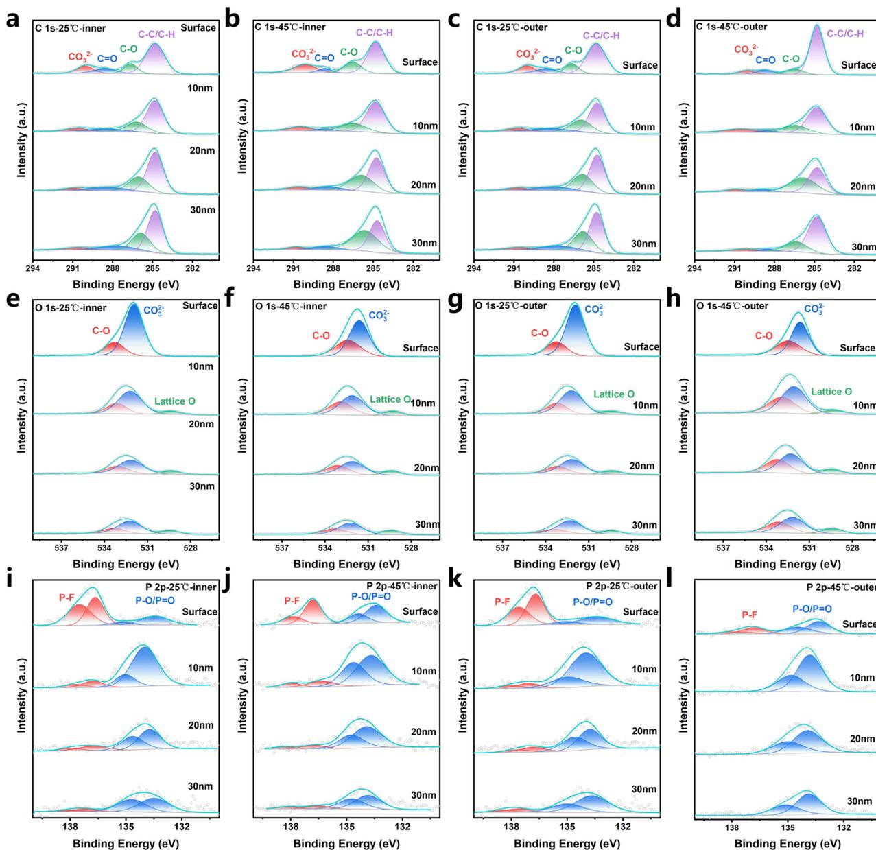
Fig. 5 XPS depth profiles of inner and outer anodes at 25 °C and 45 °C: (a–d) C 1s, (e–h) O 1s, and (i–l) P 2p.
