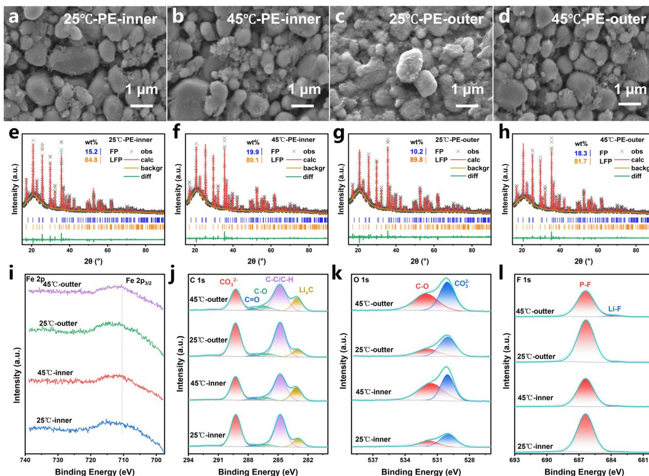
**Fig. 3** SEM images of inner cathode (a) at 25 °C and (b) at 45 °C, outer cathode (c) at 25 °C and (d) at 45 °C. XRD Rietveld refinement patterns of inner cathode (e) at 25 °C and (f) at 45 °C, outer cathode (g) at 25 °C and (h) at 45 °C. XPS spectra of (i) Fe 2p, (j) C 1s, (k) O 1s, (l) F 1s for inner and outer cathodes at 25 °C and 45 °C.
