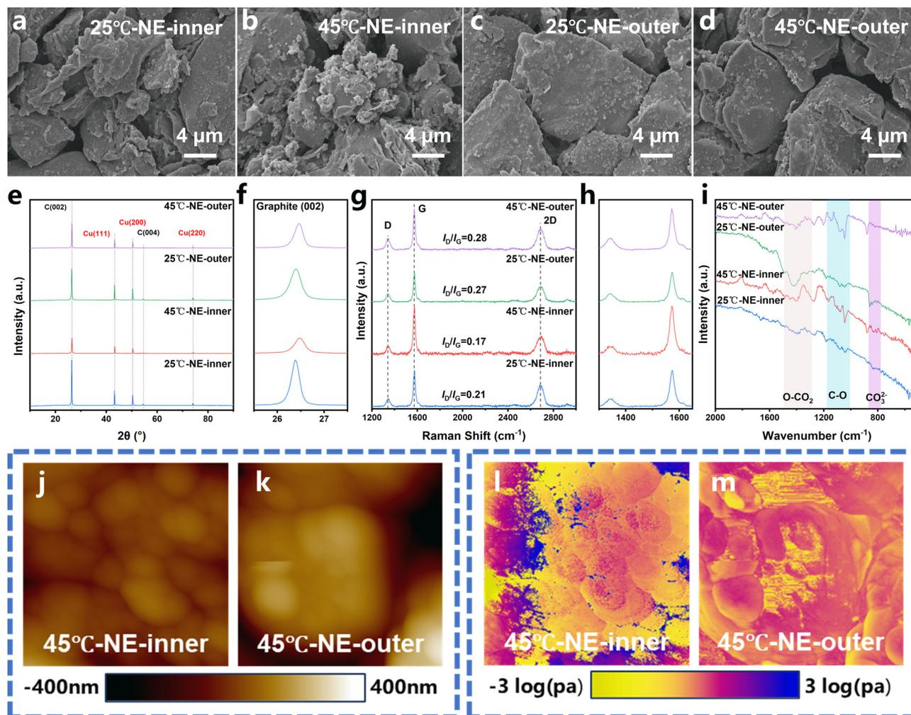
**Fig. 4** SEM images of inner anode (a) at 25 °C and (b) at 45 °C, outer anode (c) at 25 °C and (d) at 45 °C. (e and f) XRD patterns of inner and outer anode at 25 °C and 45 °C. (g and h) Raman spectra of inner and outer anode at 25 °C and 45 °C. (i) FTIR spectroscopy of inner and outer anode at 25 °C and 45 °C. AFM analysis of 2D height images for (j) inner anode and (k) outer anode. 2D Young's modulus for (l) inner anode and (m) outer anode.
