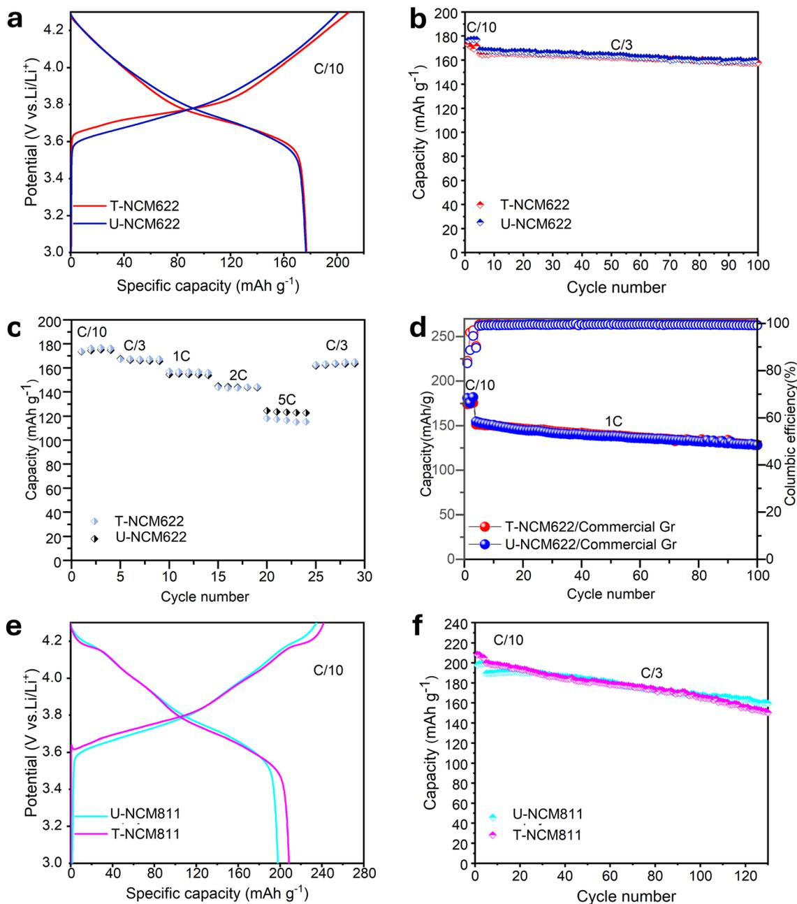
**Fig. 3** Electrochemical performance evaluation of upcycled materials. (a) First cycle voltage profiles, (b) cycling stability, and (c) rate performance of U-NCM622 compared with those of pristine T-NCM622. (d) Full cell cycling stability of the U-NCM622 sample compared with that of pristine T-NCM622 at 1C. (e) First cycle voltage profiles and (f) cycling stability of U-NCM 811 compared with those of pristine T-NCM811.
