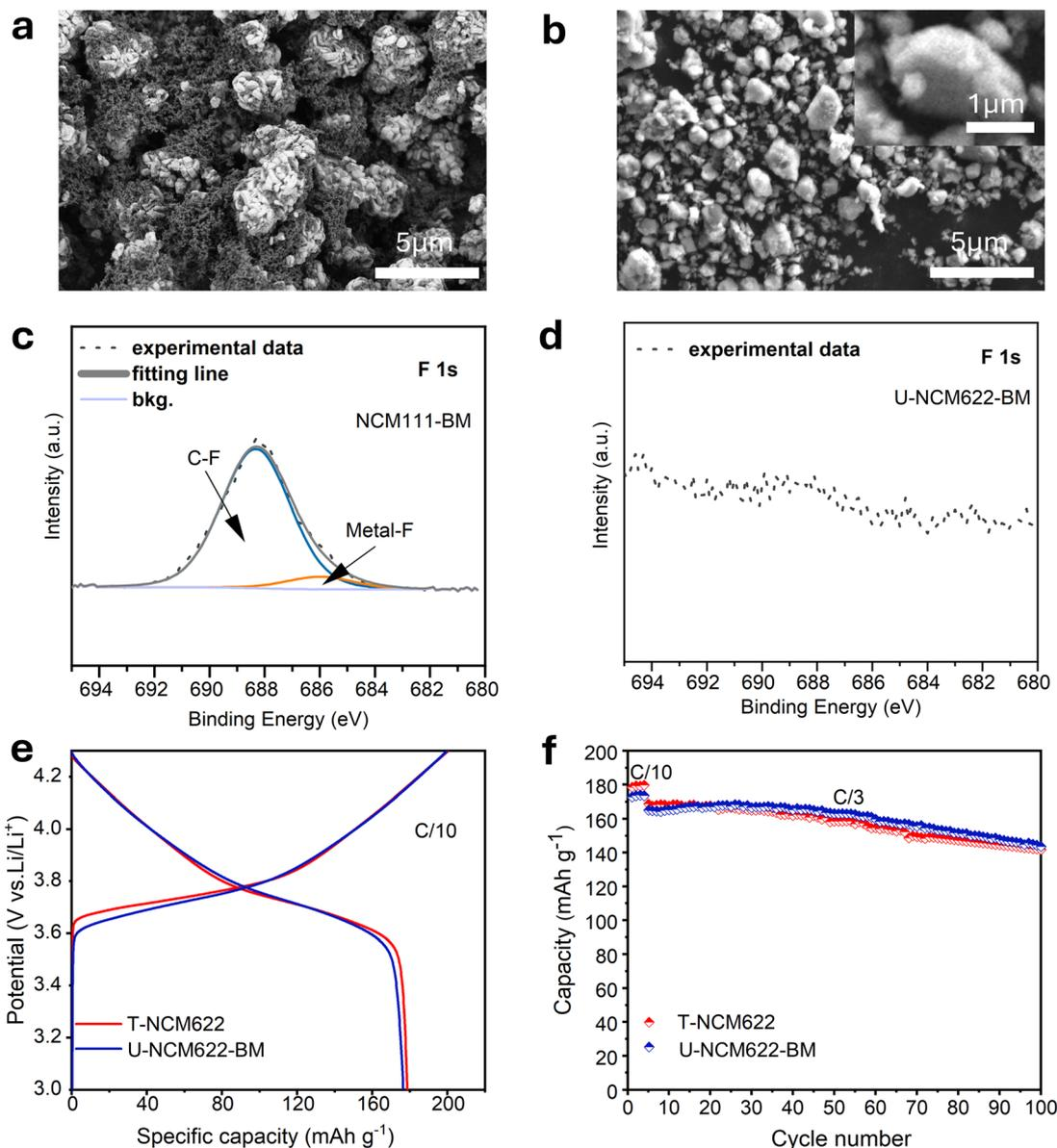
**Fig. 4** Feasibility demonstration. SEM images of (a) spent NCM111 black mass and (b) upcycled NCM622 (U-NCM622-BM) using NCM111 cathode black mass from an EV battery as raw materials. XPS data of fluorine for (c) spent NCM111 black mass and (d) U-NCM622-BM to indicate the removal of the binder from the recovered cathode through a selective upcycling process. (e) First cycle voltage profile and (f) cycling stability for U-NCM622-BM, compared with those of T-NCM622.
