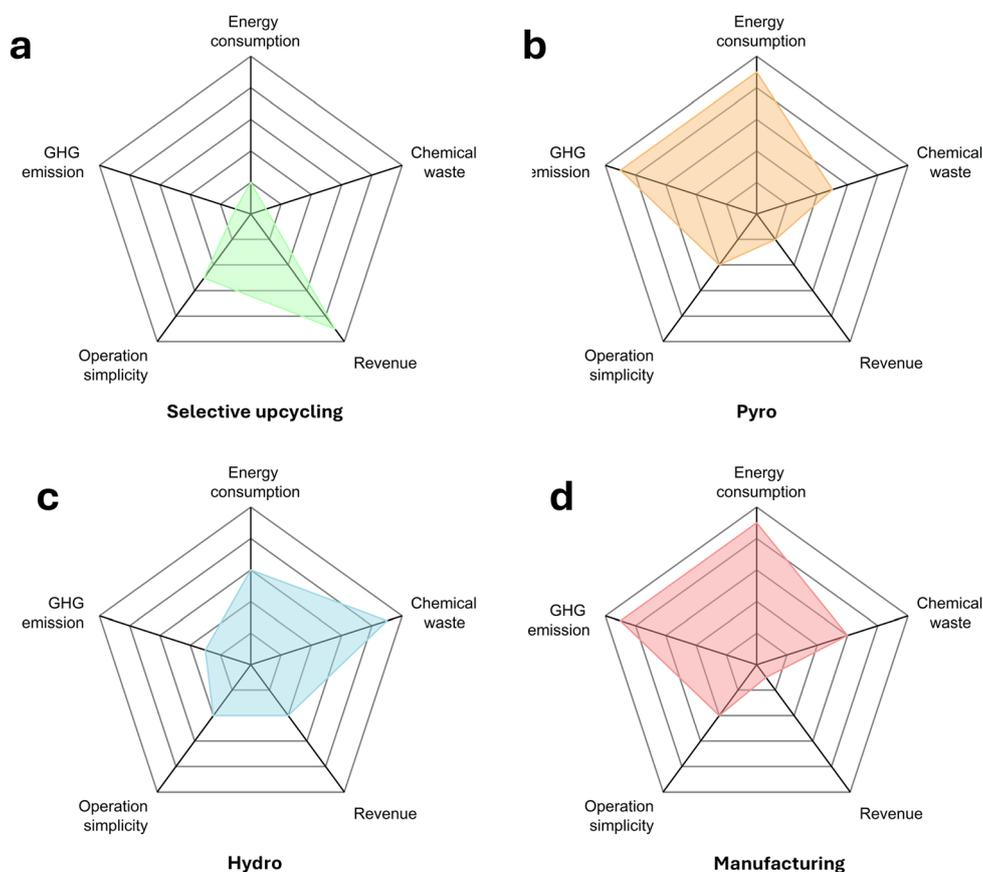
**Fig. 5** Economic and environmental analysis. Schematic of this work (“selective upcycling”), pyrometallurgical (“Pyro”), and hydrometallurgical (“Hydro”) methods, as well as cathode production (“Manufacturing”) from virgin materials mining. Spider charts comparing various features of (a) this work, (b) Pyro, (c) Hydro, and (d) cathode production methods.
