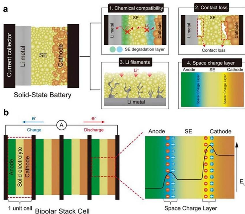
**Fig. 4** Schematic representation of a solid-state battery and bipolar stack cell: (a) various issues at electrode/electrolyte interface; (b) space charge layers in a bipolar stack cell (black line indicates the unequal Li chemical potential of the electrode/electrolyte interface of the cell during charge).<sup>73</sup> Copyright 2022, Springer.
