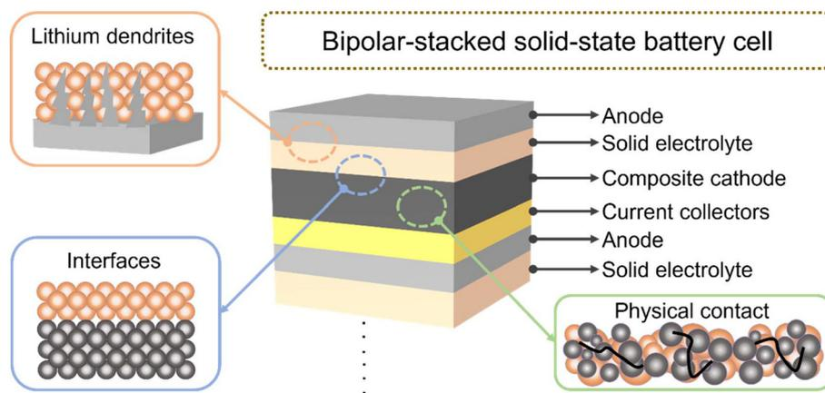
**Fig. 1** Schematic representation of a bipolar ASSB. Insets are magnified sections that highlight the three main challenges faced by solid-state batteries with metal anodes: inhomogeneous metal deposition, formation of a blocking interface and contact loss on electrochemical cycling.
