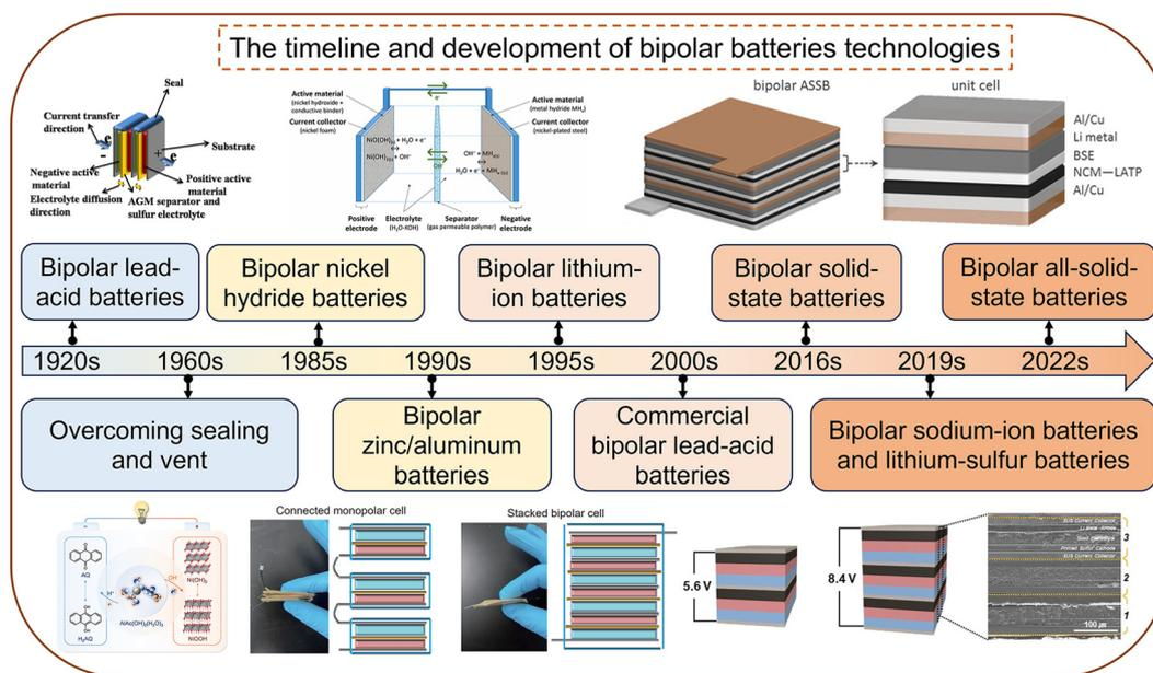
Fig. 2 Timeline and development of emerging bipolar battery technologies.<sup>52–57</sup> (1, Copyright 2017, Wiley-VCH; 2, Copyright 2022, Elsevier; 3, Copyright 2018, Wiley-VCH; 4, Copyright 2024, American Chemical Society; 5, Copyright 2022, Springer; 6, Copyright 2019, Wiley-VCH).
