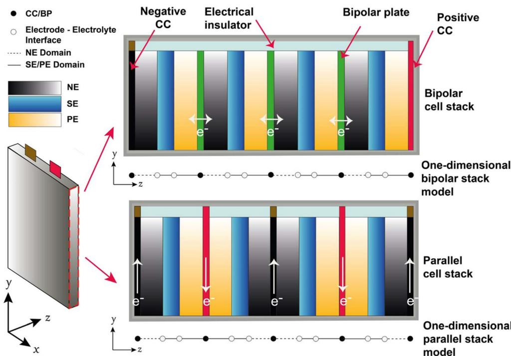
**Fig. 3** Configurations of the bipolar (top) and parallel stack (bottom) inside the pouch. In a bipolar stack, the electrical current flows from one unit cell to the adjacent unit cell through the BP, whereas in a parallel stack, the electrical current flows in-plane along the CC to the external tabs.<sup>59,60</sup> Copyright 2020, the Electrochemical Society.
