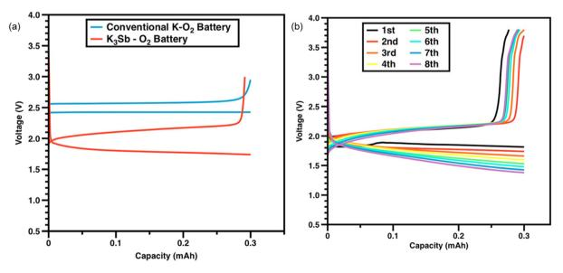
Fig. 12 (a) Galvanostatic discharge/charge profiles of a conventional  $K-O_2$  battery and a  $K_3Sb-O_2$  battery. (b) Cycling performance of the  $K_3Sb-O_2$ battery. Reproduced with permission from ref. 84. Copyright 2015 American Chemical Society.
