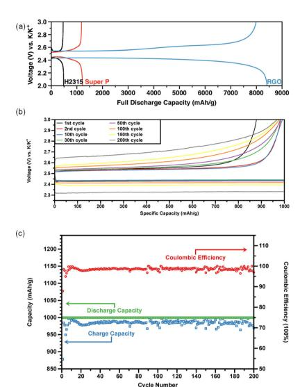
Fig. 9 (a) Discharge capacities related to the first cycle of carbon fiber electrodes (H2315 Freudenberg FCCT SE & Co. KG), Super P and rGO electrodes; (b) GCD of rGO electrodes upon cycling, and (c) cycling stability of the rGO electrode at 1000 mA g<sup>-1</sup> current rate. Reproduced with permission from ref. 75. Copyright 2016 American Chemical Society.
