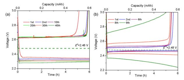
Fig. 4 Galvanostatic discharge-charge voltage profiles of K-O<sub>2</sub> batteries (a) with and (b) without a Nafion-K<sup>+</sup> membrane for various cycles. Reproduced with permission from ref. 63. Copyright 2014 American Chemical Society.
