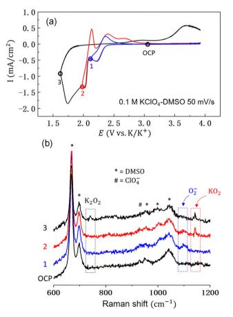
Fig. 7 (a) CV recorded in O<sub>2</sub>-saturated 0.1 M KClO<sub>4</sub> in DMSO electrolyte. (b) Surface-enhanced Raman spectra of the Au electrode at different cut-off potentials and open-circuit potential (OCP). The blue curve corresponds to a cut-off potential of 2.12 V (1), the red to 1.98 V (2), and the black to 1.60 V vs. K/K+ (3). Reproduced with permission from ref. 69. Copyright 2024 The Royal Society of Chemistry.
