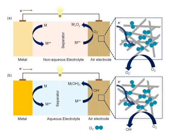
Fig. 2 Schematic illustration of (a) a metal-O<sub>2</sub> cell in a non-aqueous system and (b) metal-air cell with aqueous electrolyte.
