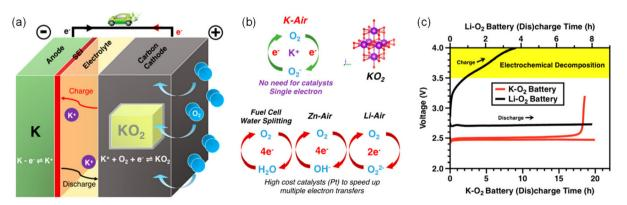
Fig. 3 (a) Schematic illustration of a K-O<sub>2</sub> battery and the discharge process in K-O<sub>2</sub> batteries. (b) Oxygen redox reaction in fuel cell water splitting, Zn-air, Li-air and K-air batteries. (c) Comparative charge-discharge profiles of Li-O<sub>2</sub> and K-O<sub>2</sub> batteries showing the low overpotentials associated with the charge-discharge process for  $K-O_2$  batteries. Reproduced with permission from ref. 60. Copyright 2018 American Chemical Society.
