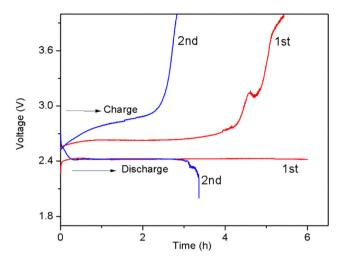
Fig. 8 Initial two continuous discharge-charge cycles of the battery at a current density of 0.16 mA cm<sup>-2</sup> in a 0.5 M KPF<sub>6</sub> electrolyte solution composed of butyl diglyme and diglyme (2:5 v/v ratio). Reproduced with permission from ref. 25. Copyright 2013 American Chemical Society.
