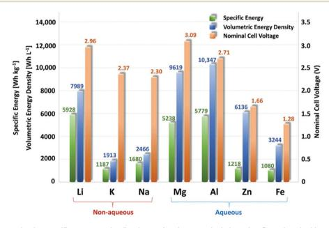
Fig. 1 Theoretical energy density, specific energy and cell voltage of various metal—air batteries. Reproduced with permission from ref. 17. Copyright 2016 WILEY–VCH Verlag GmbH & Co. KGaA, Weinheim.
