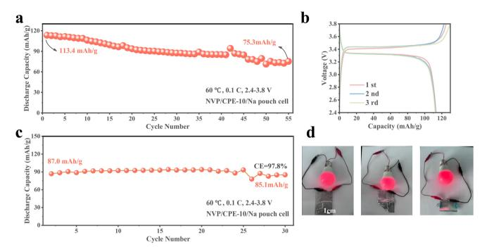
Fig. 7 (a) Cycling performance of the pouch-type all-solid-state NVP/CPE-10/Na cell at 0.1C with a cathode loading of 2.1 mg cm<sup>-2</sup>. (b) Corresponding charge-discharge curves of the pouch-type NVP/CPE-10/Na cell at different cycling stages. (c) Cycling performance of the pouchtype all-solid-state NVP/CPE-10/Na cell at 0.1C with a cathode loading of 4.0 mg cm<sup>-2</sup>. (d) Lighting test of the NVP/CPE-10/Na pouch cell under repeated bending and folding.
