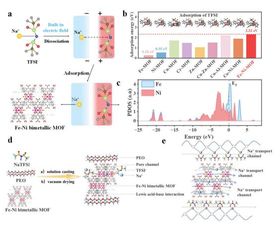
Fig. 1 (a) Detailed depiction of the dissociation and adsorption mechanisms of NaTFSI. (b) Theoretical calculations that screen the adsorption energy of TFSI<sup>-</sup> on reported and representative single-metal and bimetallic MOFs. (c) DFT-calculated DOS of MOF(Fe-Ni). (d) Schematic diagram of CPE synthesis. (e) Schematic illustration of the Fe-Ni MOF-enhanced structure of CPEs with selective and rapid Na<sup>+</sup> transport.
