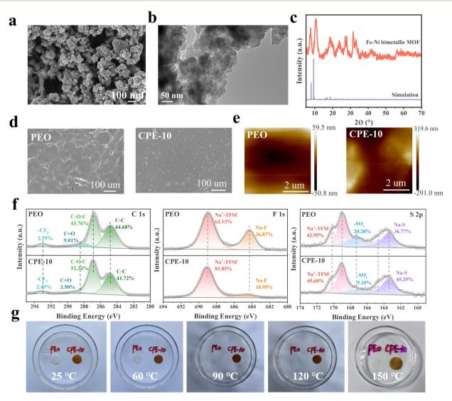
Fig. 2 (a) SEM image and (b) TEM image of the as-prepared Fe-Ni MOF powder. (c) XRD and simulated XRD patterns of the Fe-Ni MOF. (d) SEM images of PEO and CPE-10. (e) Surface morphologies of PEO and CPE-10 obtained by AFM. High-resolution XPS spectra of (f) C 1s, (g) F 1s and (h) S 2p for PEO and CPE-10 membranes. (g) Optical photographs of the states of PEO and CPE-10 membranes at 25, 60, 90, 120 and 150 °C.
