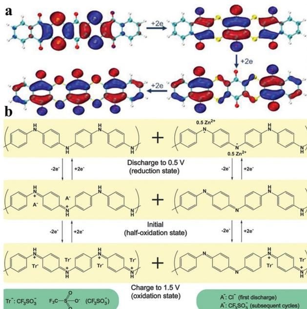
**Fig. 6** (a) HOMO plots of selected molecules/anions with different extents of reduction of BNDTH. Reproduced with permission from ref. 65. (b) The proposed redox mechanism of PANI/CFs. Reproduced with permission from ref. 66.
