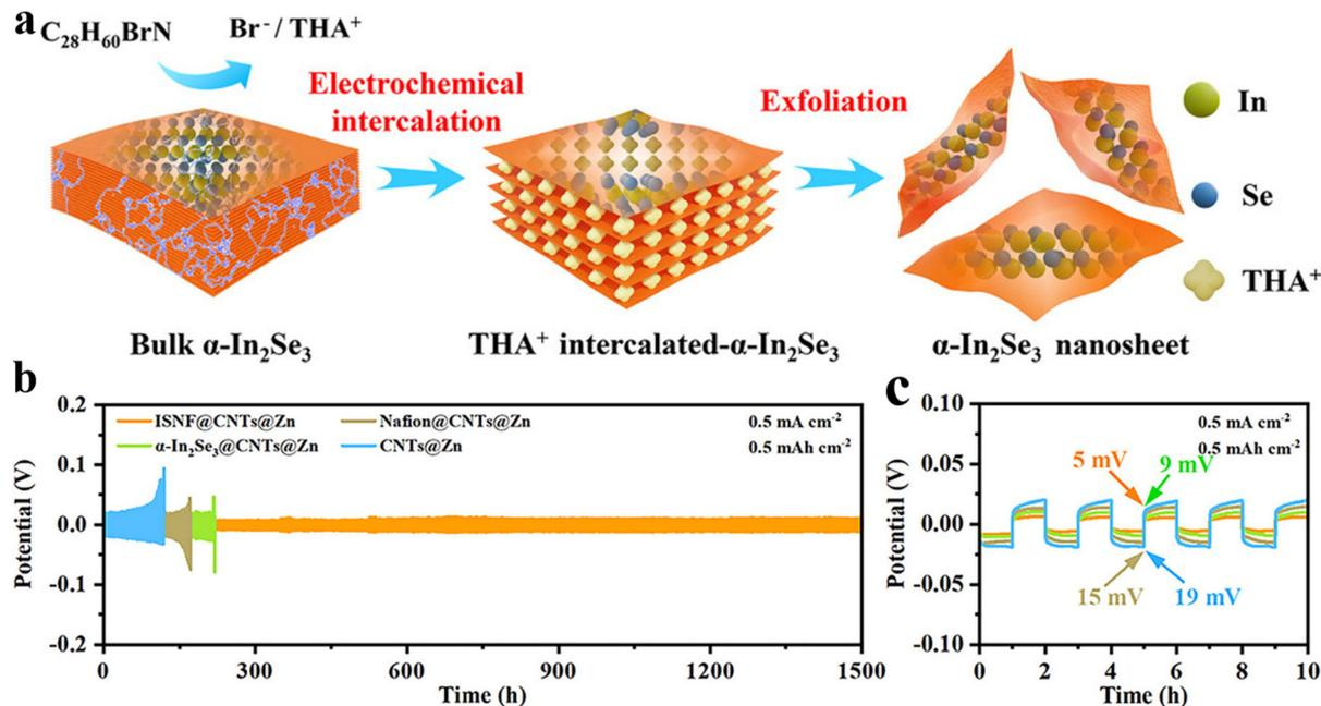
**Fig. 9** (a) Schematic illustrations of fabricating  $\alpha$ - $\text{In}_2\text{Se}_3$  nanosheets. Reproduced with permission from ref. 97. (b) Symmetric cells at  $0.5 \text{ mA cm}^{-2}$  for  $0.5 \text{ mAh cm}^{-2}$ . Reproduced with permission from ref. 97. (c) Magnified voltage–time curves. Reproduced with permission from ref. 97.
