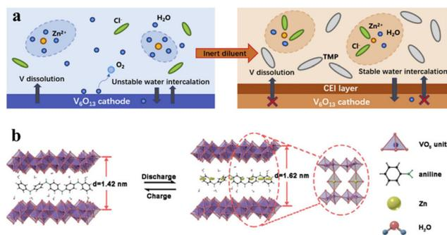
Fig. 3 (a) Schematic illustration of vanadium dissolution and CEI formation in a UWA electrolyte on a  $\text{V}_2\text{O}_5$  cathode during the electrochemical reactions. Reproduced with permission from ref. 41. (b) Schematic illustrations of zinc ion insertion/extraction of PANI100- $\text{V}_2\text{O}_5$  during the discharging/charging process. Reproduced with permission from ref. 43.
