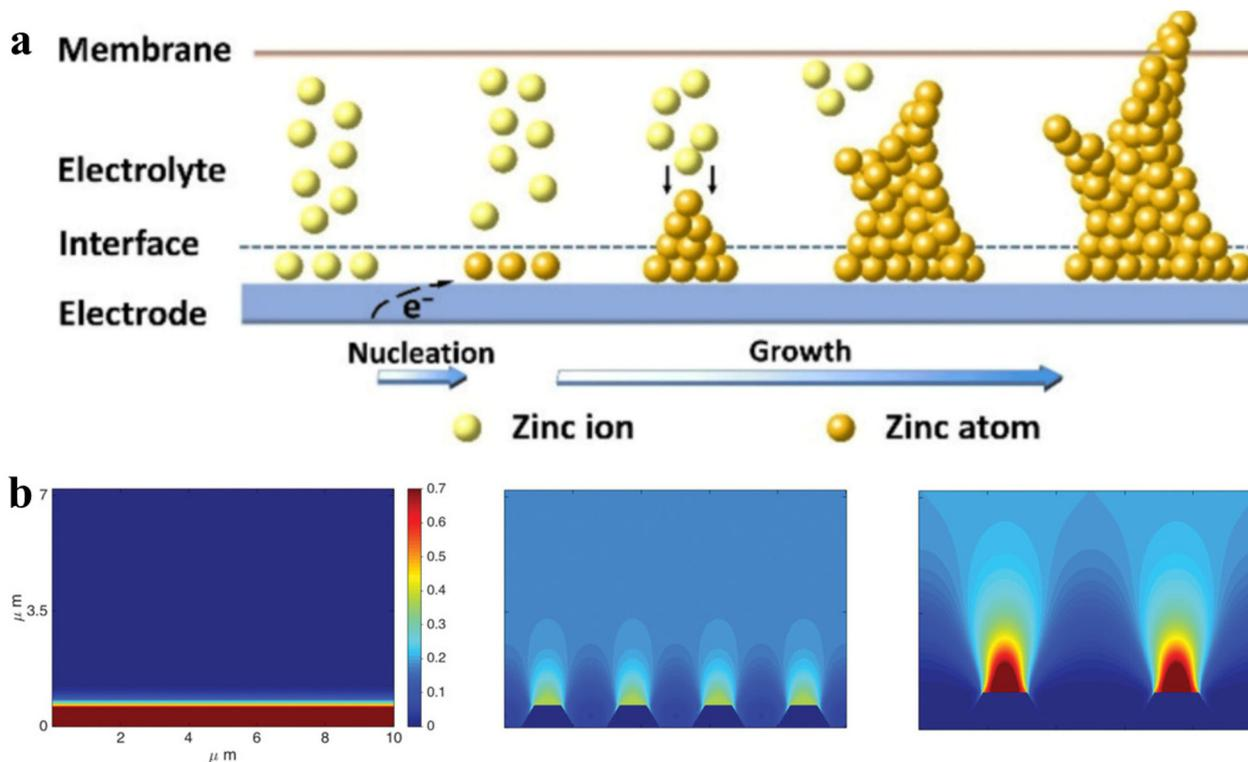
**Fig. 7** (a) Schematic diagram of dendrite growth. Reproduced with permission from ref. 72. (b) COMSOL simulation of electric field distribution on the surface of substrates with different morphologies. Reproduced with permission from ref. 75.
