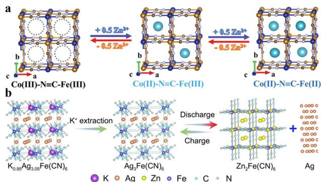
**Fig. 5** (a) Schematic illustration of reversible  $\text{Zn}^{2+}$  intercalation/deintercalation in  $\text{CoFe}(\text{CN})_6$  frameworks during the electrochemical process. Reproduced with permission from ref. 62. (b) Schematic of the energy storage mechanism in  $\text{AgHCF-3}$ . Reproduced with permission from ref. 64.
