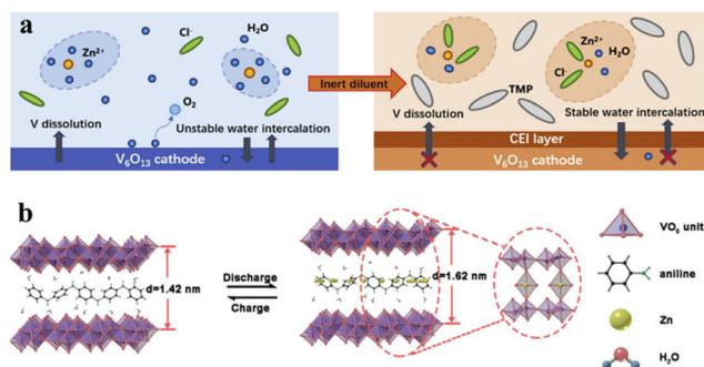
Fig. 3 (a) Schematic illustration of vanadium dissolution and CEI formation in a UWA electrolyte on a  $\text{V}_6\text{O}_{13}$  cathode during the electrochemical reactions. Reproduced with permission from ref. 41. (b) Schematic illustrations of zinc ion insertion/extraction of PANI100- $\text{V}_2\text{O}_5$  during the discharging/charging process. Reproduced with permission from ref. 43.
