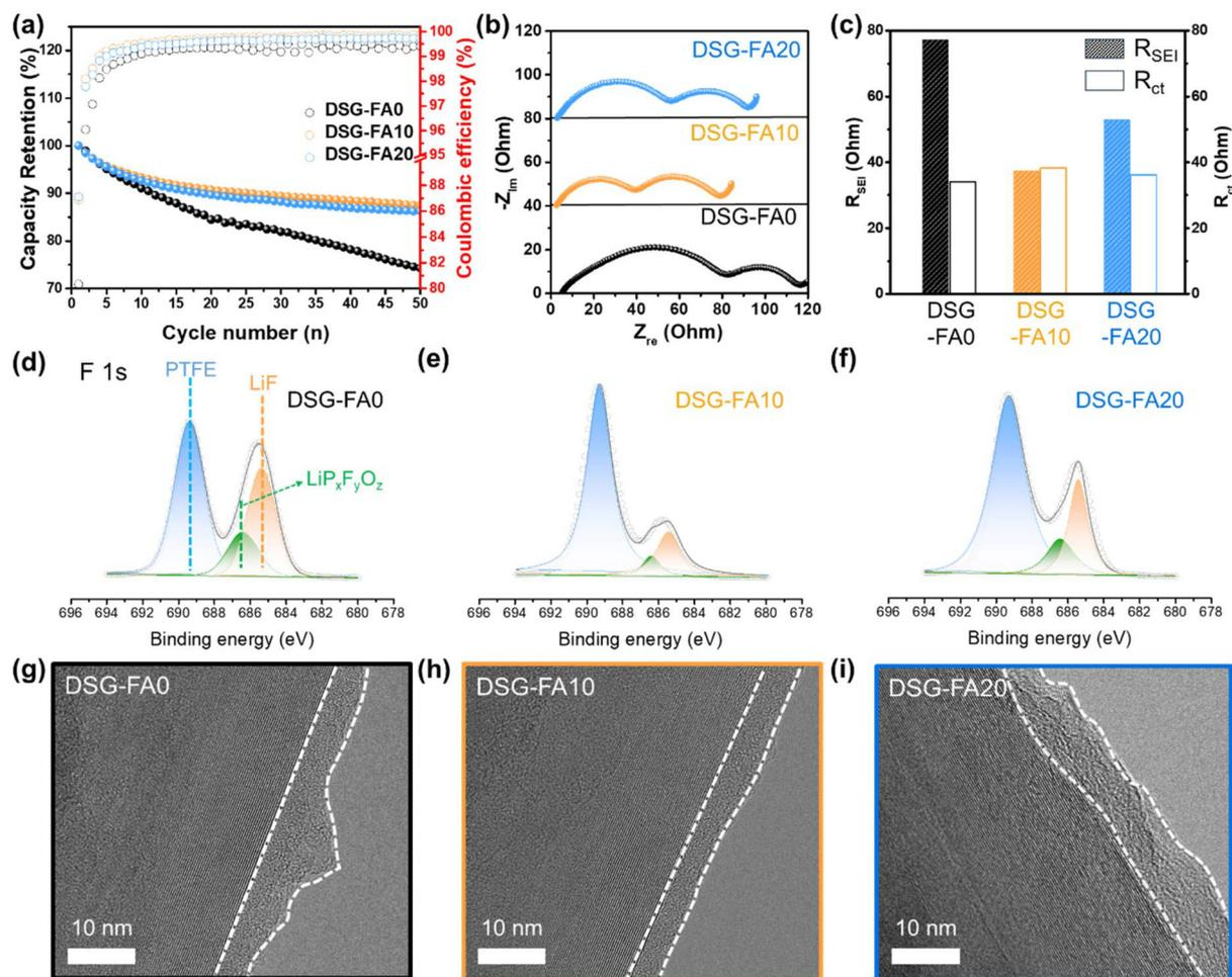
**Fig. 3** Electrochemical performances of half-cells using DSG-FA0, DSG-FA10 and DSG-FA20 anodes. (a) Cycling performances for 50 cycles. (b) Nyquist plots after 50 cycles (c)  $R_{SEI}$  and  $R_{ct}$  values corresponding to the EIS results. F 1s XPS spectra of (d) DSG-FA0, (e) DSG-FA10 and (f) DSG-FA20 after 50 cycles. TEM images of the dry-processed anode surface of (g) DSG-FA0, (h) DSG-FA10 and (i) DSG-FA20 after 50 cycles.
