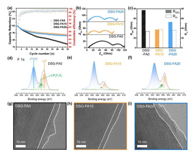
Fig. 3 Electrochemical performances of half-cells using DSG-FA0, DSG-FA10 and DSG-FA20 anodes. (a) Cycling performances for 50 cycles. (b) Nyquist plots after 50 cycles (c)  $R_{\rm SEI}$  and  $R_{\rm ct}$  values corresponding to the EIS results. F 1s XPS spectra of (d) DSG-FA10 and (f) DSG-FA20 after 50 cycles. TEM images of the dry-processed anode surface of (g) DSG-FA10 and (i) DSG-FA20 after 50 cycles.
