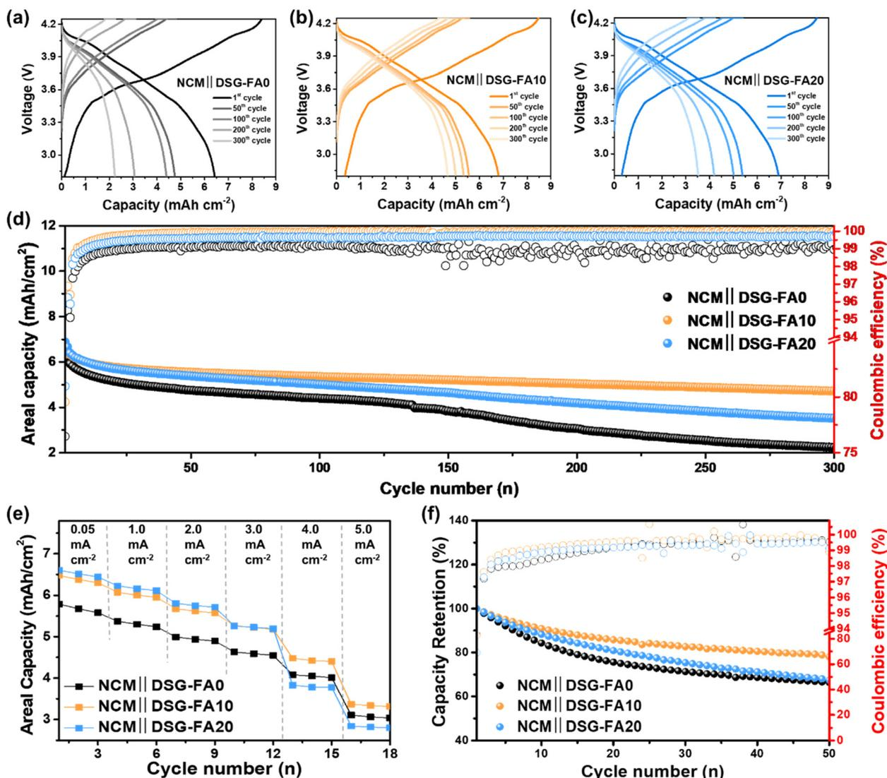
Fig. 4 Electrochemical performances of full cells under a cathode areal capacity of 6.7 mA h cm<sup>-2</sup> (anode areal capacity of 7.6 mA h cm<sup>-2</sup>) with different FA concentrations. Voltage profiles over multiple cycles for (a) NCM||DSG-FA0, (b) NCM||DSG-FA10, and (c) NCM||DSG-FA20 anodes. (d) Long-term cycling performances up to 300 cycles at 0.2 C-rate. (e) Rate capabilities measured from 0.05 to 5.0 mA cm<sup>-2</sup>. (f) High-rate cycling stability for 50 cycles at 2.0 C-rate.
