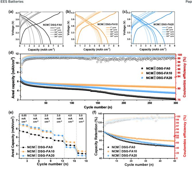
Fig. 4 Electrochemical performances of full cells under a cathode areal capacity of 6.7 mAh cm<sup>-2</sup> (anode areal capacity of 7.6 mAh cm<sup>-2</sup>) with different FA concentrations. Voltage profiles over multiple cycles for (a) NCM||DSG-FA0, (b) NCM||DSG-FA10, and (c) NCM||DSG-FA20 anodes. (d) Long-term cycling performances up to 300 cycles at 0.2 C-rate. (e) Rate capabilities measured from 0.05 to 5.0 mA cm<sup>-2</sup>. (f) High-rate cycling stability for 50 cycles at 2.0 C-rate.
