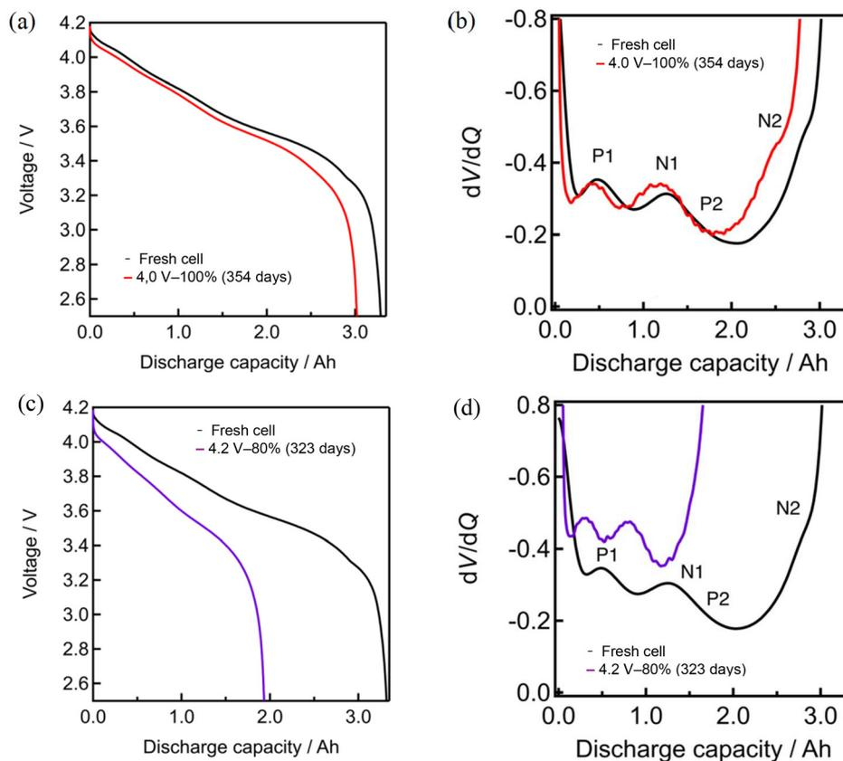
Fig. 3 0.1C discharge profiles and the corresponding  $dV/dQ$  profiles of (a and b) 4.0 V-100% (after 354 days) and (c and d) 4.2 V-80% cells (after 323 days). (a) and (c) show the discharge curves, while (b) and (d) show their derivative  $dV/dQ$  profiles in comparison with the data of the fresh cell.
