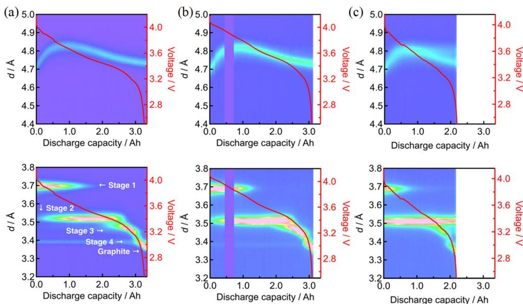
**Fig. 8** Operando neutron diffraction profiles of (a) the fresh cell and (b) 3.8 V–100% (after 476 days) and (c) 4.2 V–60% (after 428 days) aged cells during discharging at 0.1C. The layered positive 003 and negative graphite 001 reflections are shown on the upper and lower sides, respectively.
