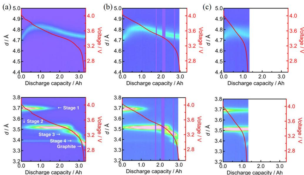
**Fig. 7** Operando neutron diffraction profiles of (a) the fresh cell and (b) 4.0 V–100% (after 476 days) and (c) 4.2 V–80% (after 323 days) aged cells during discharging at 0.1C. The layered positive 003 and negative graphite 001 reflections are shown on the upper and lower sides, respectively.
