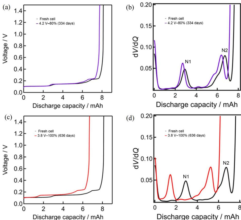
**Fig. 11** Discharge profiles of negative electrodes in half cells at 0.02C derived from (a and b) 4.2 V–80% and (c and d) 3.8 V–100% cells. (a) and (c) show the discharge curves, while (b) and (d) show their derivative  $dV/dQ$  profiles in comparison with the data of the fresh cell. Peaks N1 and N2 show the same transitions as those shown in Fig. 3 and 4.
