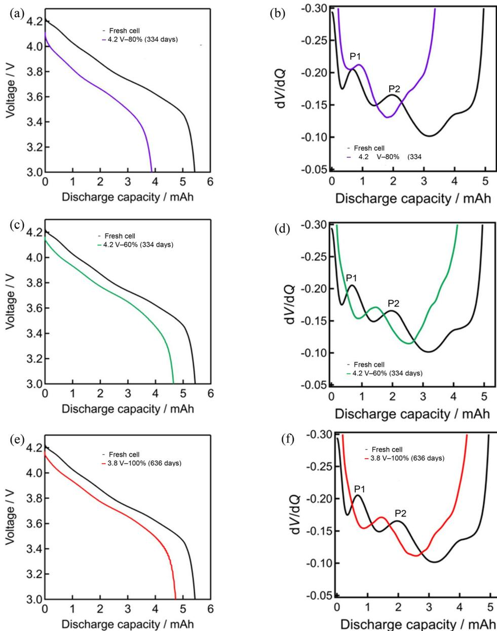
**Fig. 10** Discharge profiles of positive electrodes in half cells at 0.02C derived from (a and b) 4.2 V–80%, (c and d) 4.2 V–60%, (e and f) 3.8 V–100% cells. (a), (c) and (e) show the discharge curves, while (b), (d) and (f) show their derivative  $dV/dQ$  profiles in comparison with the data of the fresh cell. Peaks P1 and P2 show the same transitions as those shown in Fig. 3 and 4.
