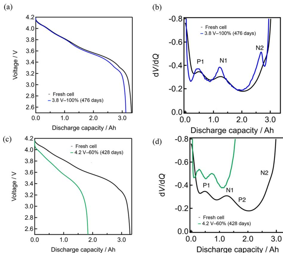
**Fig. 4** 0.1C discharge profiles and the corresponding dV/dQ profiles of (a and b) 3.8 V-100% (after 476 days) and (c and d) 4.2 V-60% cells (after 428 days). (a) and (c) show discharge curves, while (b) and (d) show their derivative dV/dQ profiles in comparison with the data of the fresh cell.
