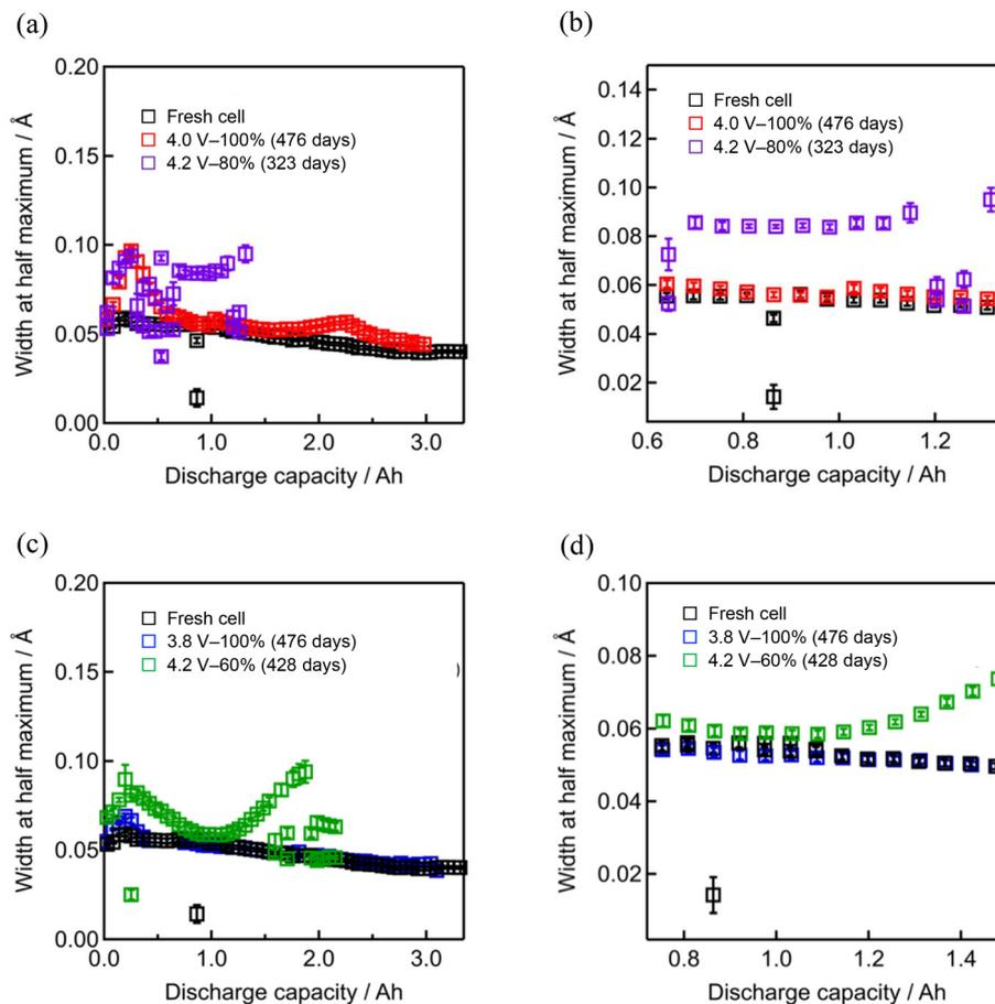
**Fig. 9** Full width at half maximum of layered positive 003 reflection obtained during operando neutron diffraction at 0.1C. (a and b) 4.0 V–100% after 476 days and 4.2 V–80% after 323 days; (c and d) 3.8 V–100% after 476 days and 4.2 V–60% after 428 days. (b) and (d) show the enlarged view of (a) and (c), respectively.
