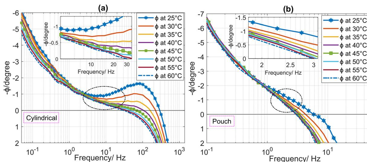
**Fig. 3** Bode plot indicating phase shift at multiple temperatures under SOC = 70% (a) cylindrical cell phase difference and showing temperature dependence as an insert, (b) phase shift for pouch cell and an insert focusing on a particular frequency region for temperature dependence, as circled in the main figure.
