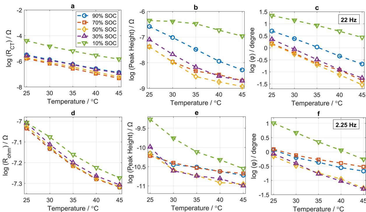
Fig. 6 Arrhenius relation for all three extracted features for both cell types at multiple SOC. (a)  $R_{CT}$  (cylindrical cell), (b) DRT peak height (cylindrical cell), (c) phase shift at 22 Hz (cylindrical cell), (d)  $R_{ohm}$  (pouch cell), (e) DRT peak height (pouch), (f) phase shift at 2.2 Hz (pouch).
