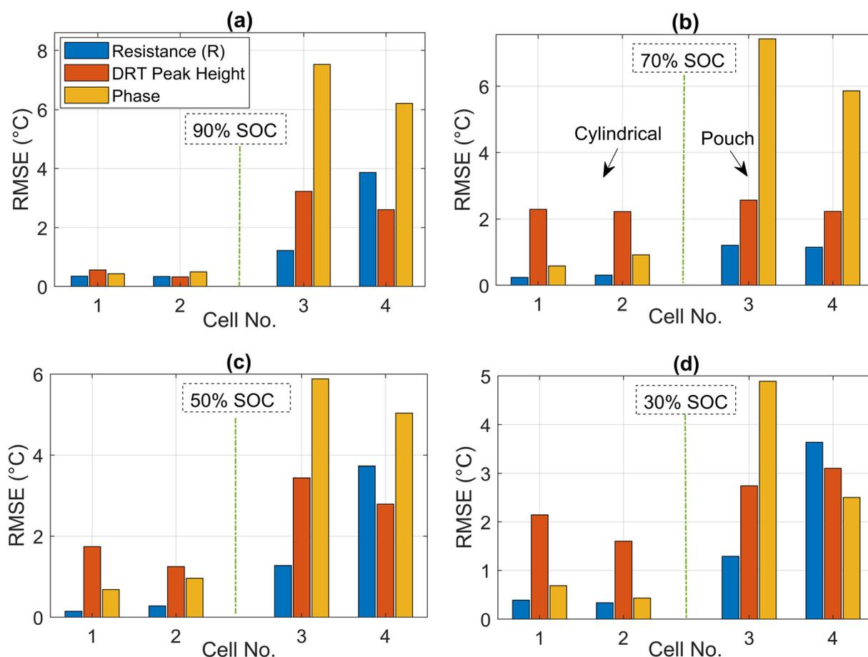
Fig. 7 Model validation using Arrhenius fit and RMSE (°C) based comparison of proposed impedance features at multiple SOCs for both cell types, (a) validation at 90% SOC, (b) 70% SOC, (c) 50% SOC, and (d) 30% SOC.
