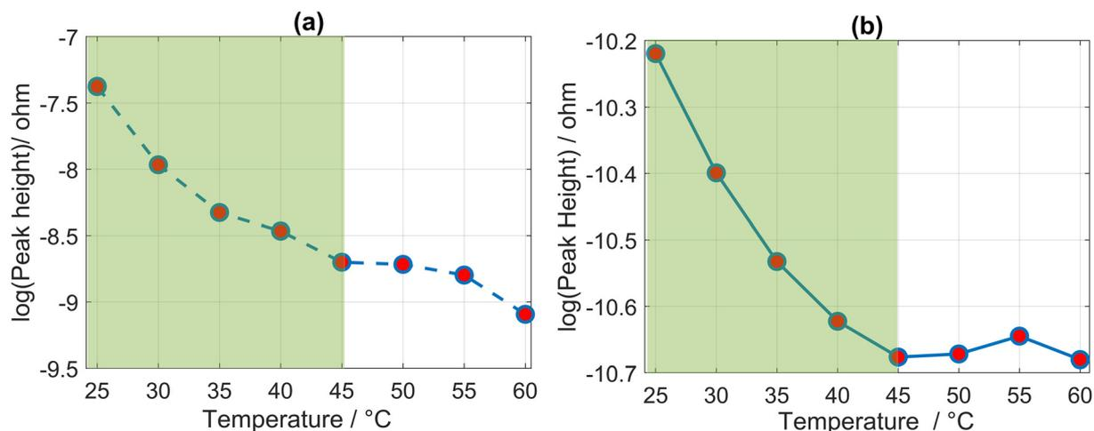
Fig. 4 Arrhenius relation based on DRT peak heights over the whole temperature range, indicating multiple linear regions at SOC 70, (a) cylindrical cell, (b) pouch cell.
